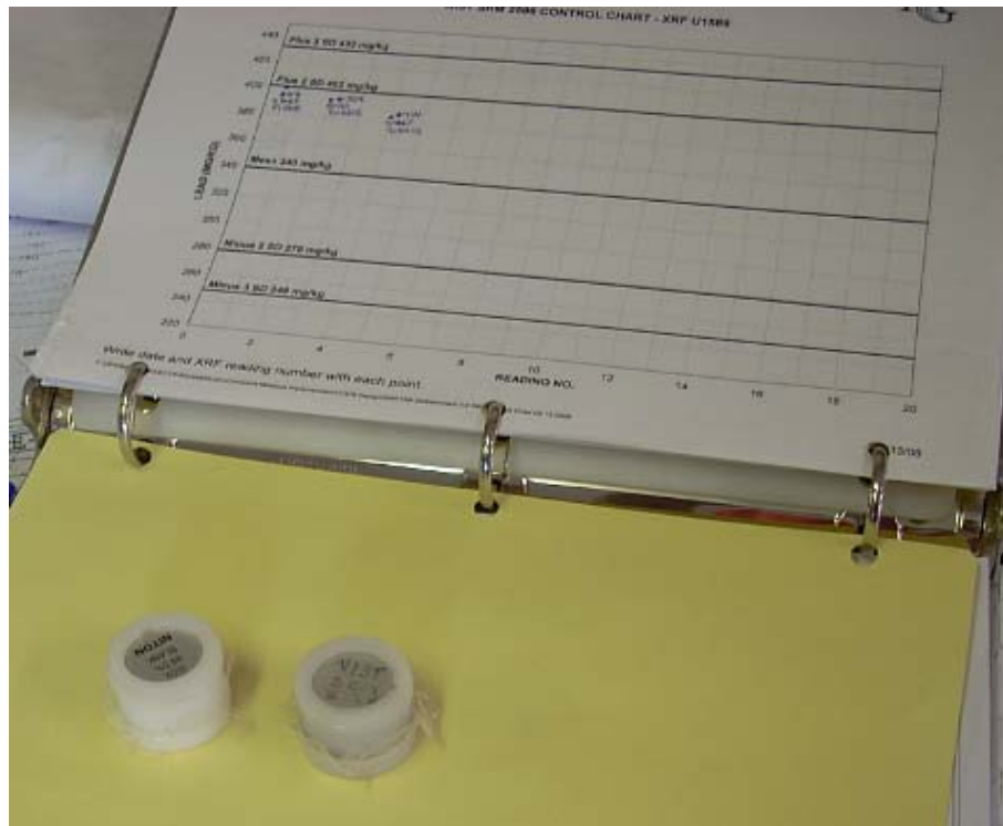
Figure 1: Example Control Chart and CRMs used for LCS
