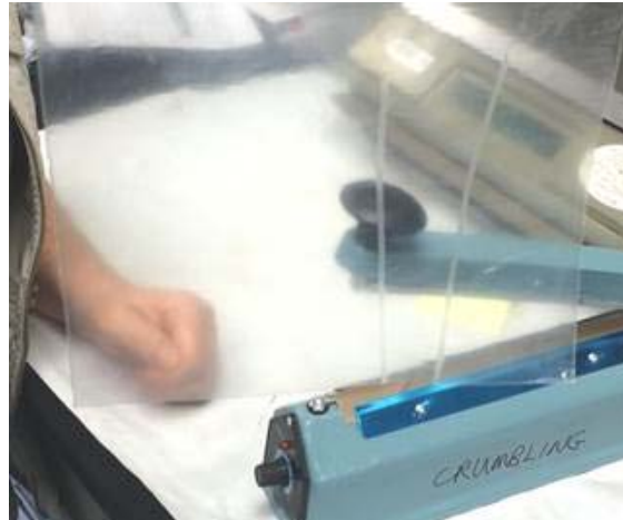
Figure 1. “Subsample tube” prepared in an interference-free sandwich “read” bag using a heat sealer.
