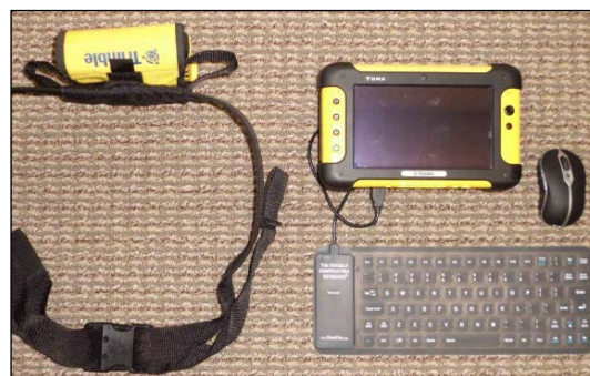
Figure 4. Trimble Yuma Rugged Tablet Computer with Pro XH Receiver Mounted on a Waist Belt
