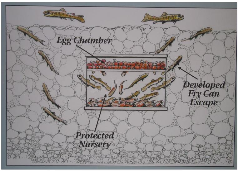
Figure 4-1. Design and Function of a Whitlock-Vibert Box
