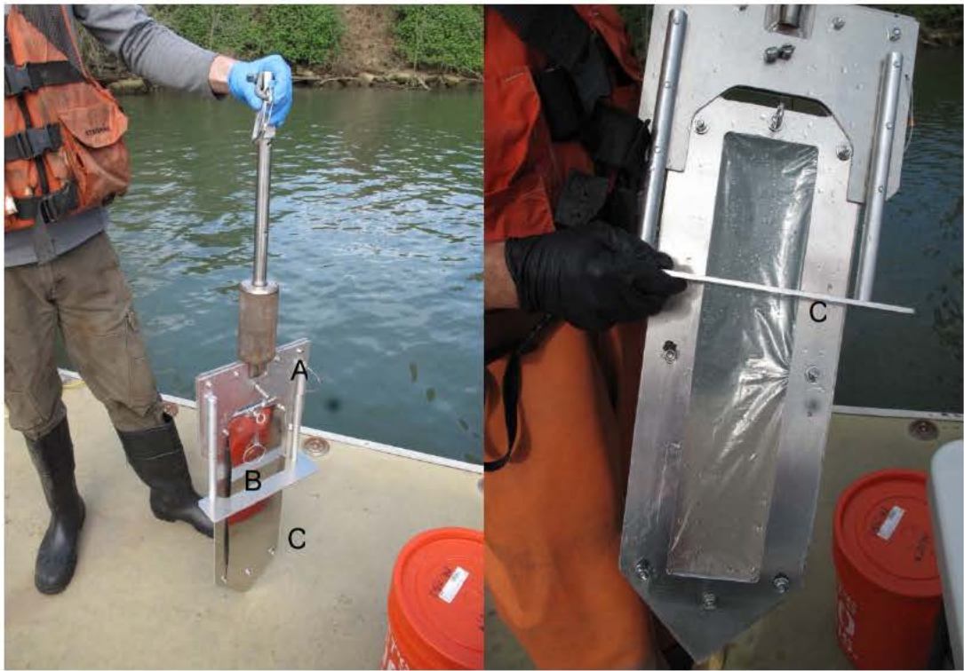
Figure 1: Passive Sampling Device Assembly
