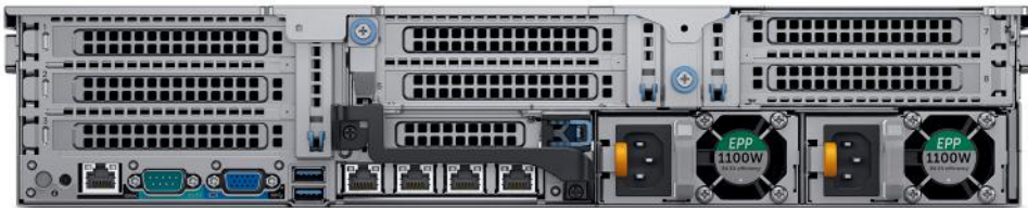
R740 Rear view - with 4x PCIe slots available with riser 2 and riser 3 blanks
