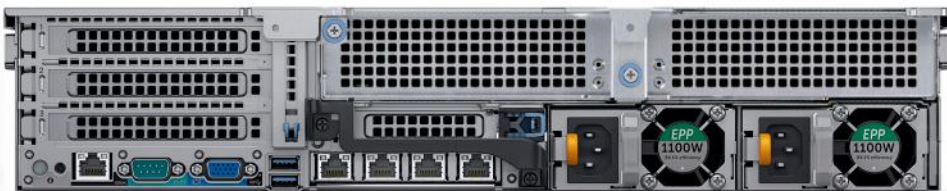
R740 Rear view - with 4x PCIe slots available with riser 2 and riser 3 blanks
