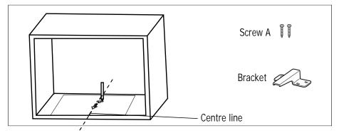
3. Remove the bottom cabinet template and fix the bracket with screw A.
