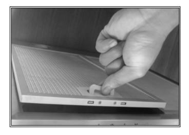
Open the front cover. Remove the grease filters by pulling down on their handles, and then pulling them upwards away from the main body of the cooker hood.
