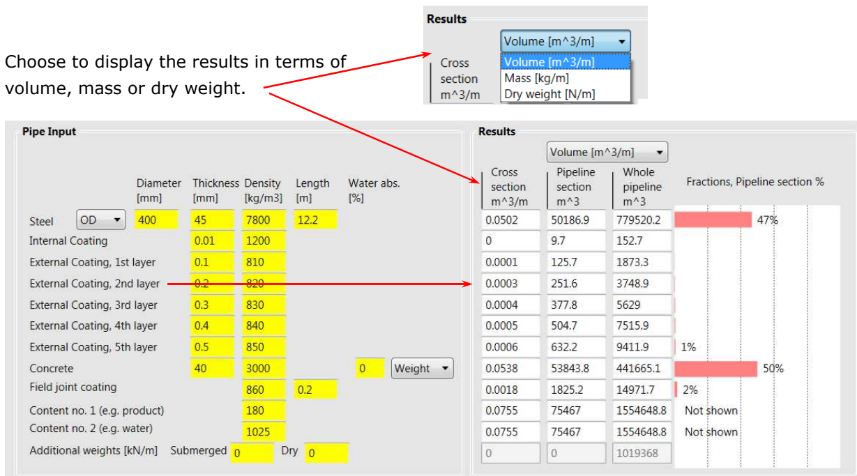
Figure 4-5 Pipe Input and results
