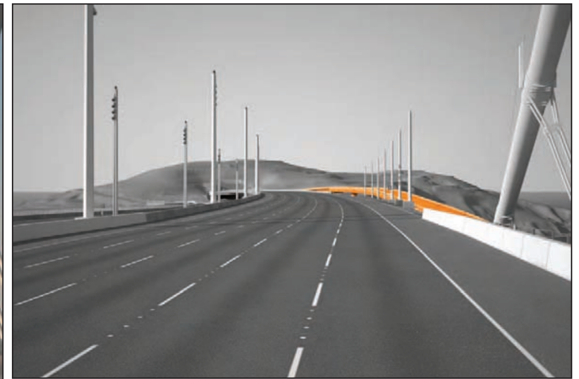
Alternative 4 Ramp Components: Orange highlighting distinguishes Alternative 4 ramp components from SFOBB East Span project components
