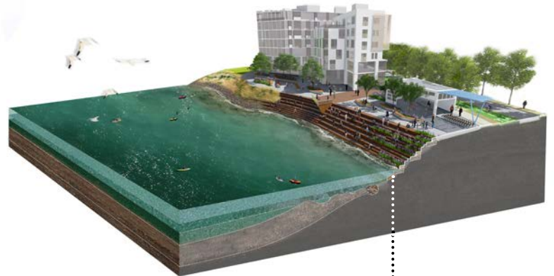
Cove 2100: +66" Relocate boardwalk at higher elevation. ....
