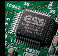
Ultra high performance ESS ES9016 DACs for all channels
