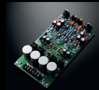
Digital/analogue boards with integrated power supply circuits
