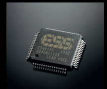
High performance ES9018 32-bit D/A converter
