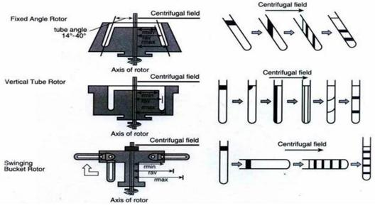
Fig: Types of centrifugation rotors
