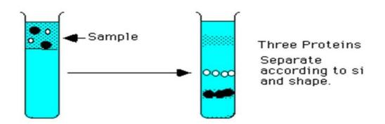
Particles can be separated by density. When the density in the solvent equals the density of the particle, the denominator of the equation equals zero and therefore velocity equals zero - the particle reaches its equilibrium density in the solvent this is called equilibrium density gradient centrifugation or isopycnic banding.
