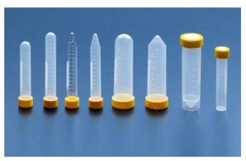
Fig: Different types of centrifugation tubes
