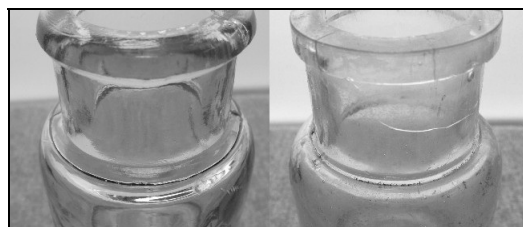
Figure 15 – V-shaped grooves in Blue machine bottles
