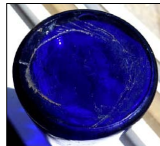
Figure 42 – Owens machine base (eBay)
