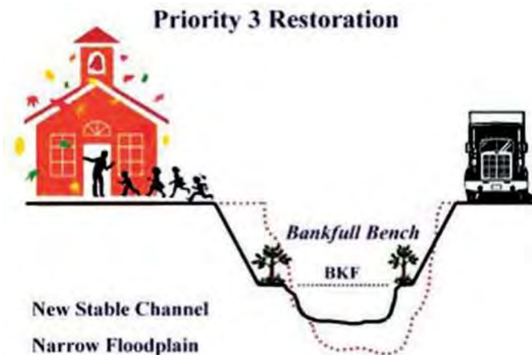
Figure 6.7: Conceptual cross section of Priority 3 restoration (Doll et al,2003)
