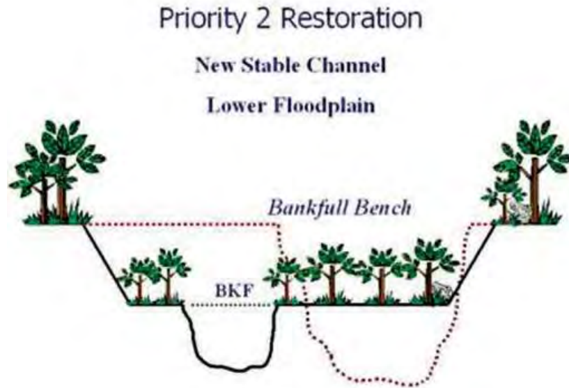
Figure 6.6: Conceptual cross section of Priority 2 restoration (Doll et al,2003)
