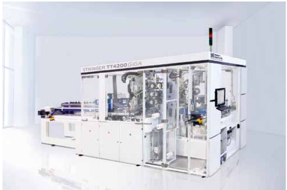
Teamtechnik's TT4200 GIGA platform can achieve an annual throughput of 130 MW on the same footprint that a machine with 30 MW could be installed only a few years ago.
