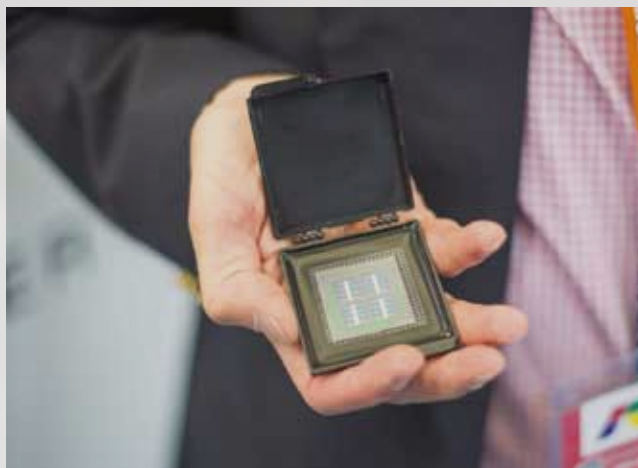
"This is a commercially produced cell with the perovskite material on top."
