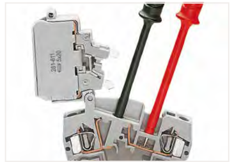
Measuring current between jumper slot and separate test slot.
