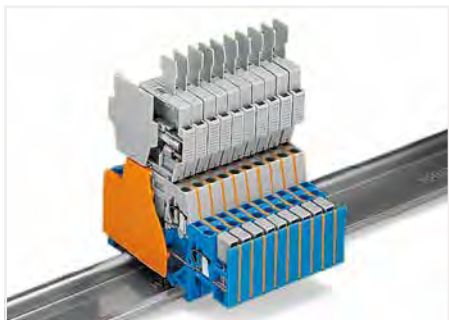
When double-deck terminal blocks are used with a fuse plug (6 mm wide) in the receptacle (top) level, the extra width of the 280 Series (5 mm wide) can be compensated for via intermediate plates (1.1 mm thick). If required, this special intermediate plate still allows commoning on the lower level via push-in adjacent jumpers (280-402).
