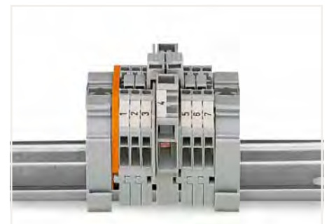
Commoning from 6 mm 2 /10 AWG (282 Series) to 1.5 mm 2 /16 AWG (279 Series) rail-mount terminal blocks via step-down jumpers.
