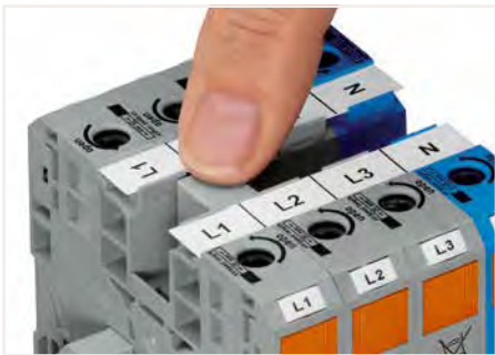
Commoning (35 mm 2 ): Commoning adjacent terminal blocks using a centrally positioned push-in jumper. Use an operating tool to remove the conductor.
