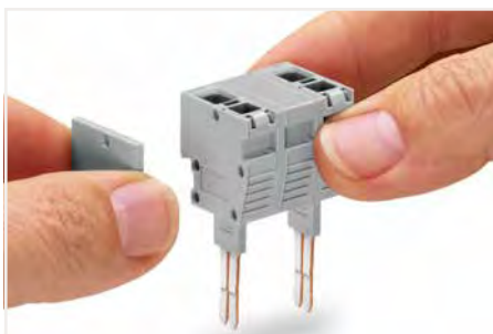
Snapping test plug and spacer modules (each with a spacer plate) together to assemble a multi-pole test plug module (max. 10 poles) for 10 mm terminal block width.
