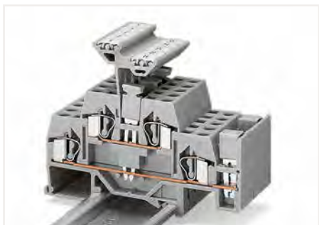
A vertical jumper commons the upper and lower decks, creating a 4-conductor commoned through terminal block in one housing. Two adjacent terminals may be commoned together on the same deck using a push-in adjacent jumper.
