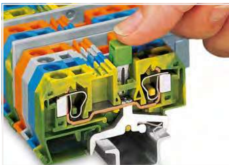
Commoning ground conductor terminal blocks with through terminal blocks is possible in one direction only (via rear side of terminal block) using adjacent jumpers. WAGO recommends using yellow-green adjacent jumpers in addition to the required marking of these blocks.
