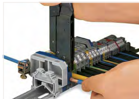
Insert the fixed peg into the upper operating slot, then hook the movable clamp into the lateral operating slot. The contact is fully opened by pressing the handles together until they engage.
