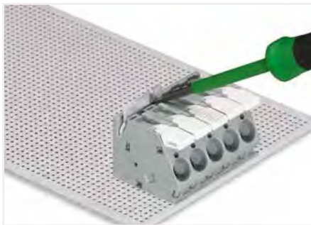
Push jumper bar down firmly using a screwdriver until it hits the backstop – 2706 and 2716 Series.
