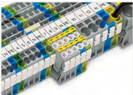
Insulation stops reliably prevent the insulation of thin conductors from being clamped. Protective warning covers identify terminal blocks that carry voltage even when the main switch is open.
