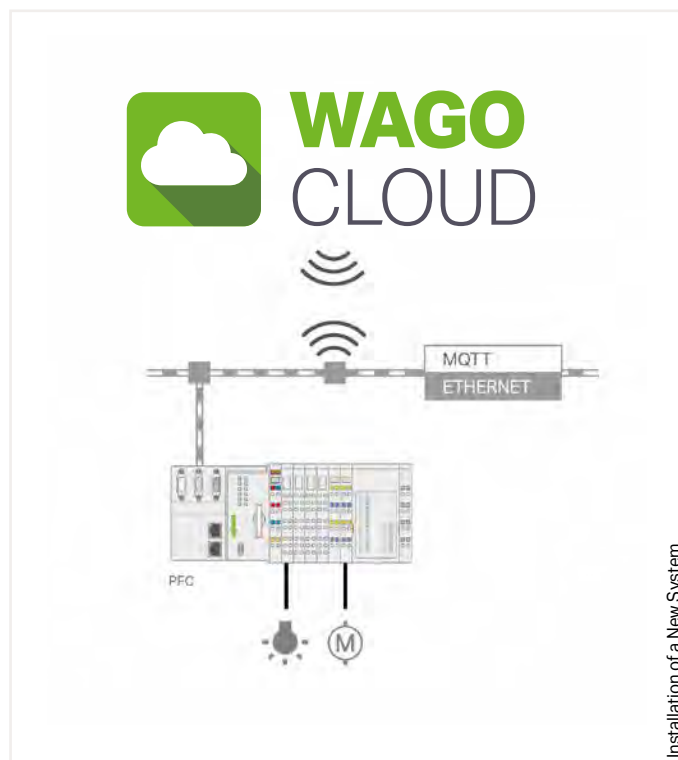
Retrofit – Installation Parallel to Existing Systems
