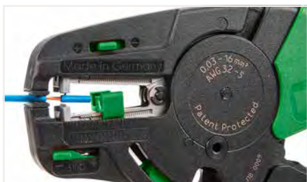
Partially stripping a conductor
