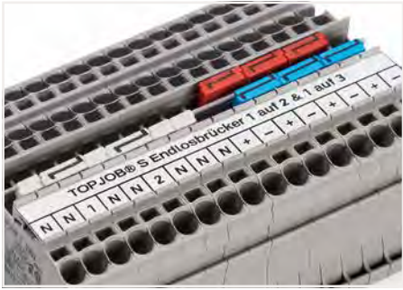
The 1-to-3 adjacent jumper for continuous commoning enables every other terminal block to be commoned. For example, positive and negative potentials can be accommodated alongside each other.
