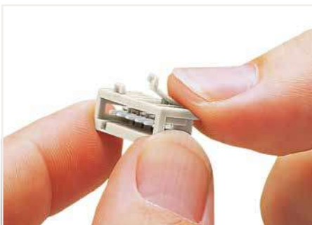
Coding a male header – fitting coding key(s).
