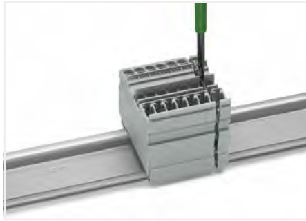
Open the assembly by laterally sliding a block via operating tool (3.5 x 0.5 mm blade).
