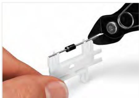
Cutting component to the proper length
