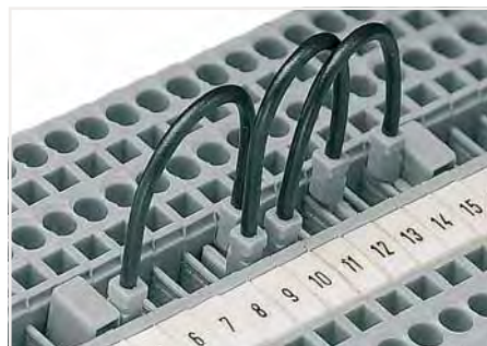
The 280/775/780 and 281/776/777/781 Series Terminal Blocks accept two wire jumpers, allowing the use of commoning chains. Furthermore, the 280/769/775/780/880 and 281/776/777/781 Series allow both a wire jumper and an adjacent jumper to be simultaneously plugged into a same terminal block.
