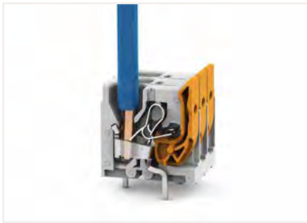
Solid conductors allow direct push-in termination; fine-stranded conductors can only be connected with lever open – 2606 Series
