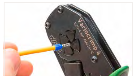
Insert the ferruled conductor into the crimping station.
