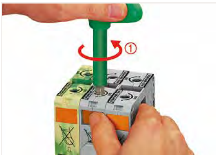
Conductor termination (50, 95 and 185 mm 2 ) – step 1 Rotate the T-wrench counter-clockwise to the stop ①. Next, push in the orange locking tab. The clamp is locked open for hands-free wiring.
