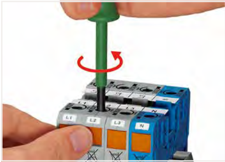
Conductor termination (35 mm 2 ) – step 1 Rotate the operating tool (5.5 mm blade width) counter-clockwise. Next, push in the orange locking tab. The clamp is locked open for hands-free wiring.
