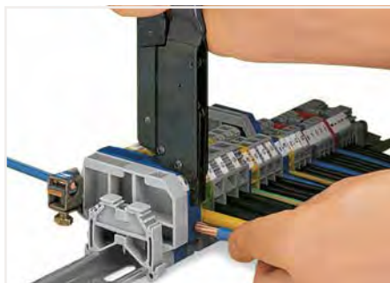
When operating the handles beyond the locked position, the ratchet allows the tool to open and be removed from the terminal block.
