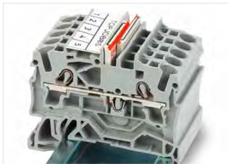
Orient the staggered jumpers' red stripes on the inside. Insert the staggered jumper and push down until it hits the backstop.
