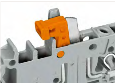
Disconnect/test terminal block with pivoting knife disconnect and mechanical interlock – knife disconnect in open position
