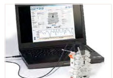
Interface Configuration software, with 750-923 USB Communication Cable
