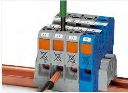
Conductor termination (35 mm 2 ) – step 2 Insert a stripped conductor into the clamping unit until it hits the backstop. Hold in this position.
