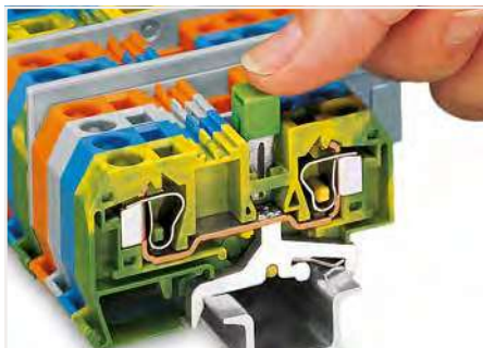
Commoning ground conductor terminal blocks through terminal blocks is possible in one direction only (via rear side of terminal block) using adjacent jumpers. WAGO recommends using yellow-green adjacent jumpers in addition to the required marking of these blocks.
