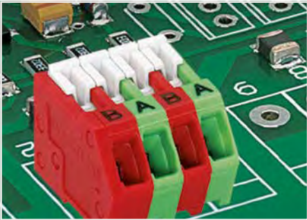
Directly marked at the factory
