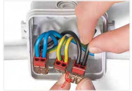
Removal: Hold conductor to be removed and twist alternately left and right while pulling the connector.
