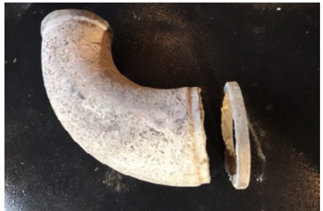
Fig. 2. A high powered Shotcrete pump sheared an un-rated elbow reducer. Luckily, no one was injured.
