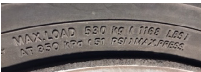
Fig. 1. Similar appearing tires may have very different load ratings.
