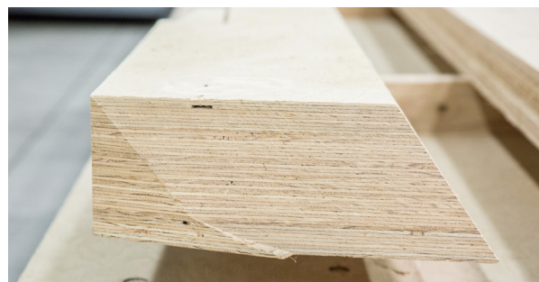
Figure 6. A mass plywood panel made by Freres Lumber Company. Photo Photo courtesy of Freres Lumber Company https://www.flickr.com/photos/frereslumber/44238527941/in/album-72157671902713093/
