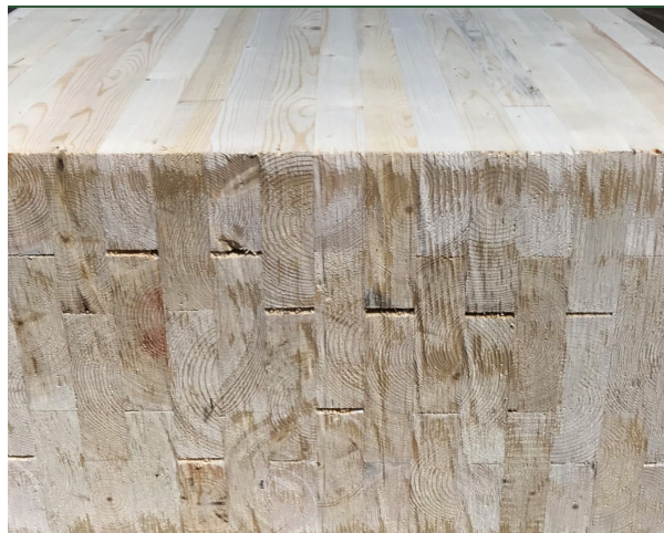
Figure 3. Glulam cross-section. Photo courtesy of ThinkWood ( https://www.thinkwood.com/mass-timber/glulam )
