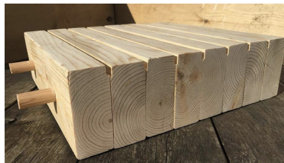
Figure 5. Dowel-laminated timber sample. Photo courtesy of Fast+Epp ( https://www.fastepp.com/concept-lab/material/dowel-laminated-timber-dlt-4/ )
