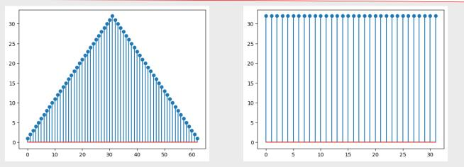
In this problem we convolved two rectangular signals with non-zero samples in the range  $0 \le n < 32$  to get a result that had non-zero samples in the range  $0 \le n < 64$ .
