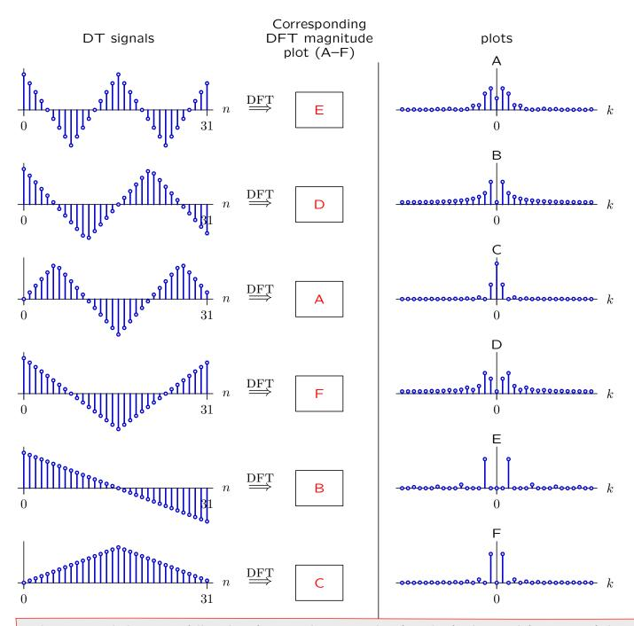
The top signal shows two full cycles of a triangle wave. Therefore the fundamental frequency of the triangle wave falls at k = 2. There could also be harmonics of k = 2 (i.e., at k = 4, 6, 8, ...).  $\rightarrow$  plot E The next two signals show 1.5 full cycles of a triangle wave. Therefore the magnitude will peak between
