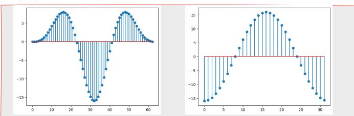
In this problem, one cycle of a sine wave with length 32 was convolved with itself. The result was greatest when the positive half cycles of the signals overlapped (n = 16) and smallest when the positive and negative halves overlapped (n = 32).
