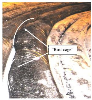
Figure 3: Cable with "bird-cage" [1]
