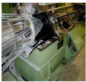
Figure 2: Wires being coated with bitumen
