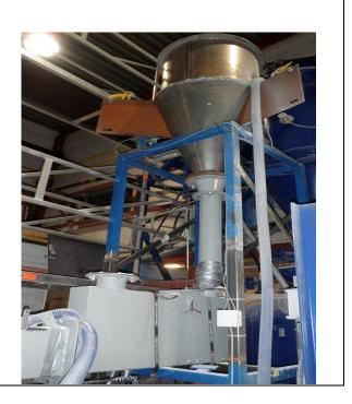
Figure 1 Experimental setup: a) initial 2012 design using bigger feeding silo, short pipe and iris valve, b) 2013 design using smaller silo, weight beam cells and standpipe concept.
