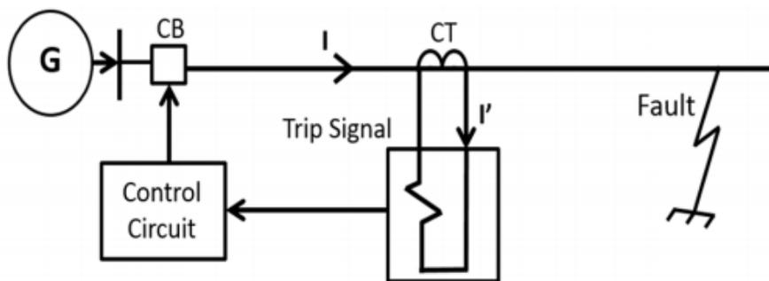
Fig 2: Representation of overcurrent relay
