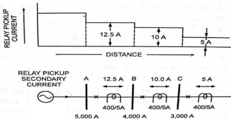
**\*\*The short ckt current along the length of protected ckt decreases with increase in distance between supply end and fault point**
