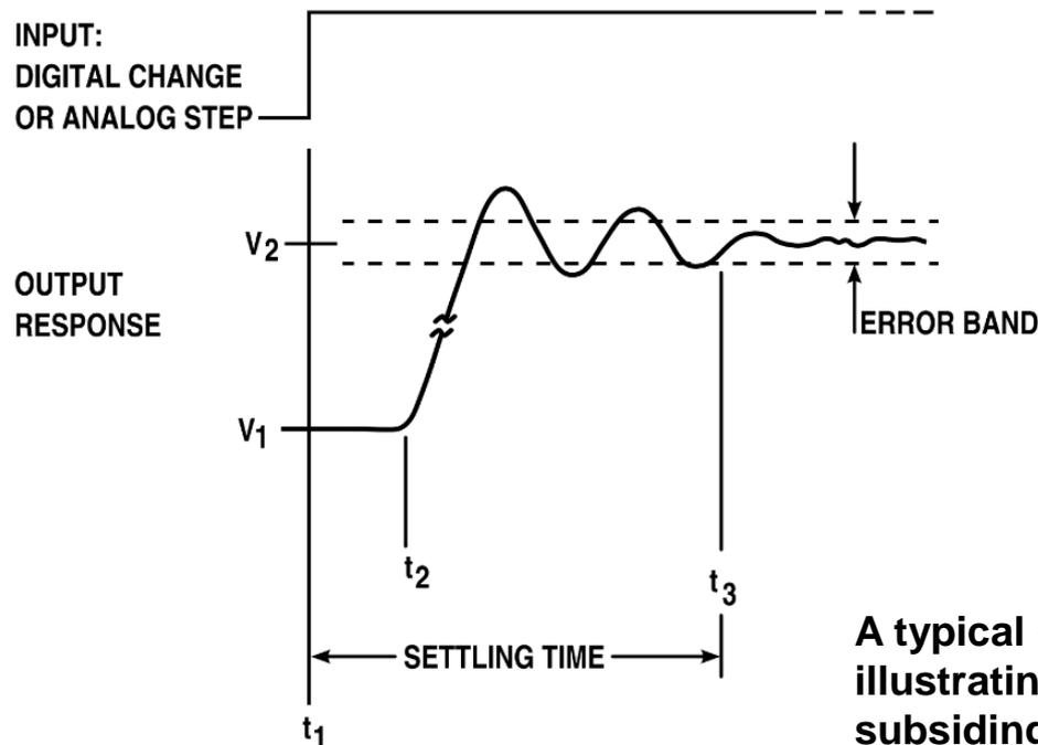
**A typical step response for a second order system, illustrating overshoot, followed by ringing, all subsiding within a settling time.**
