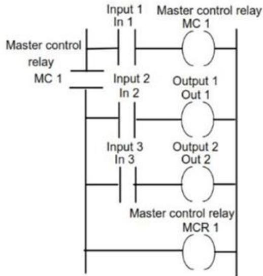
**MASTER CONTROL RELAY** – to control large number of outputs – turn on/off whole section of ladder diagram
