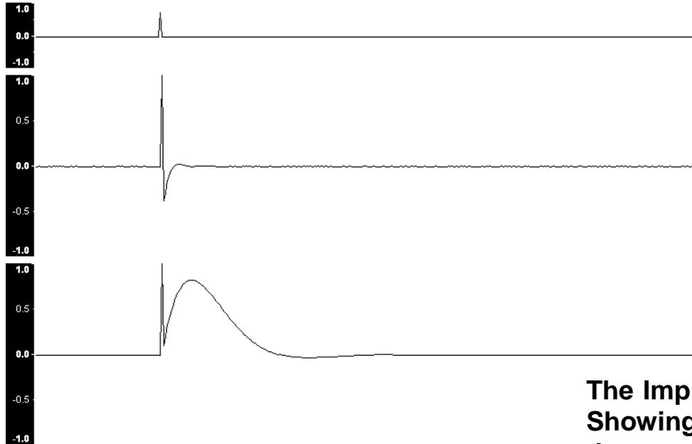
**The Impulse response from a simple audio system. Showing, from top to bottom, the original impulse, the response after high frequency boosting, and the response after low frequency boosting.**
