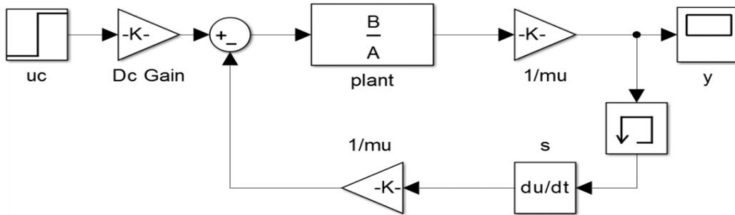
Figure c: Second order system adjustment with first order controller block diagram
