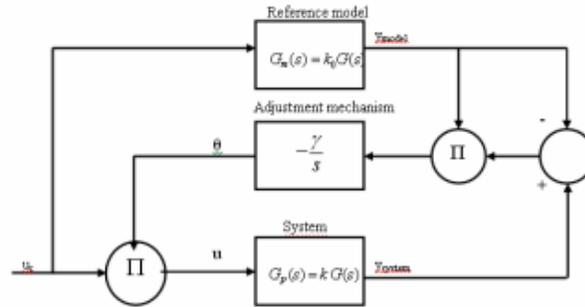
The system model for the adaptive control according to the MIT rule
