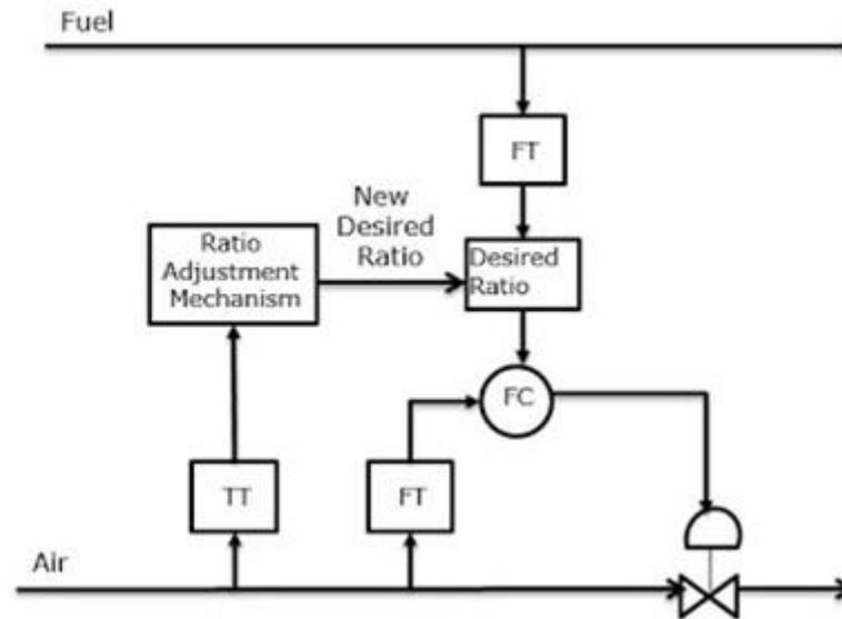
**Adaptive Ratio Control Mechanism for a Combustion System**
