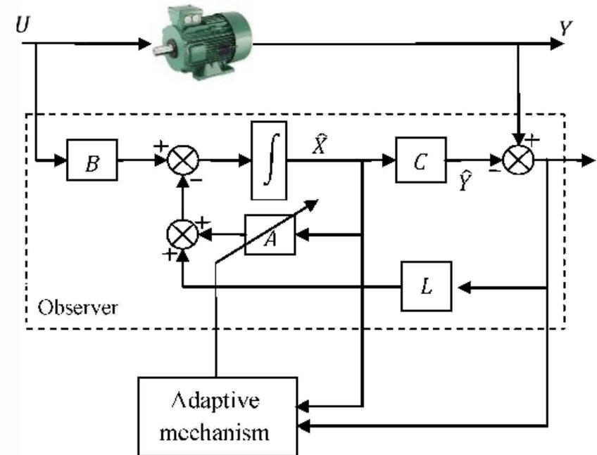
Figure 4. Structure of the adaptive Luenberger observer
