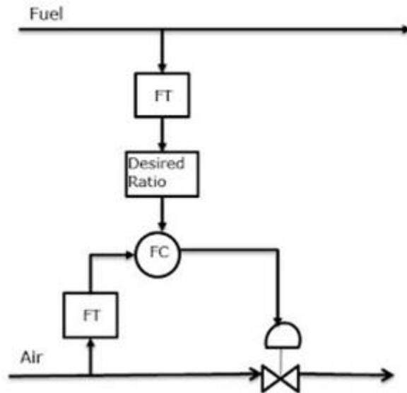
**Ratio Control for a Combustion System**
