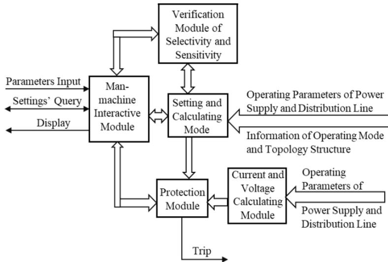
Fig 5: Adaptive protection of power supply and distribution system
