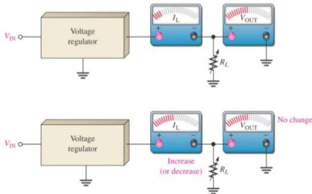
Load regulation: A change in load current (due to a varying  $R_L$ ) has practically no effect on the output voltage of a regulator (within certain limits)
