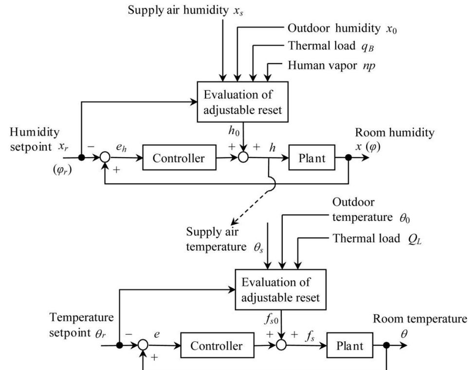
Figure 3 Overall of the combined control system
