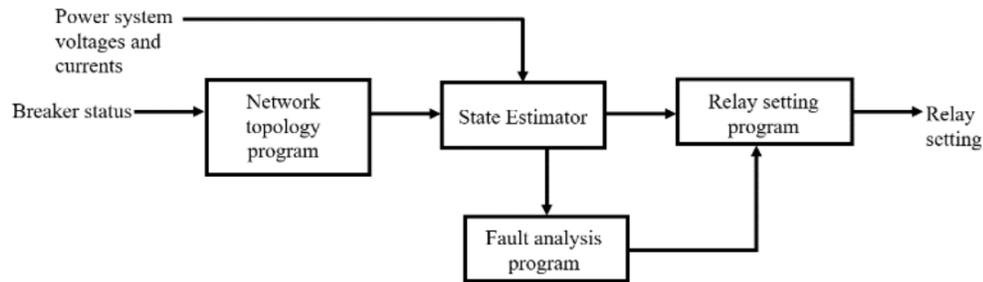
Fig 6: Block diagram of relay co-ordination software
