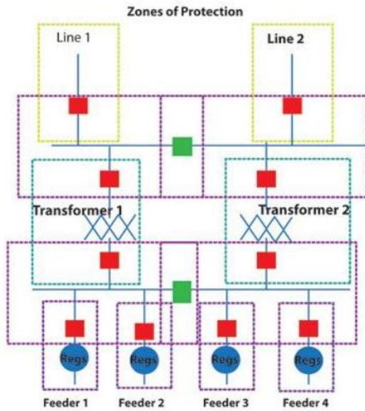
Fig : Overall structure of general protection system
