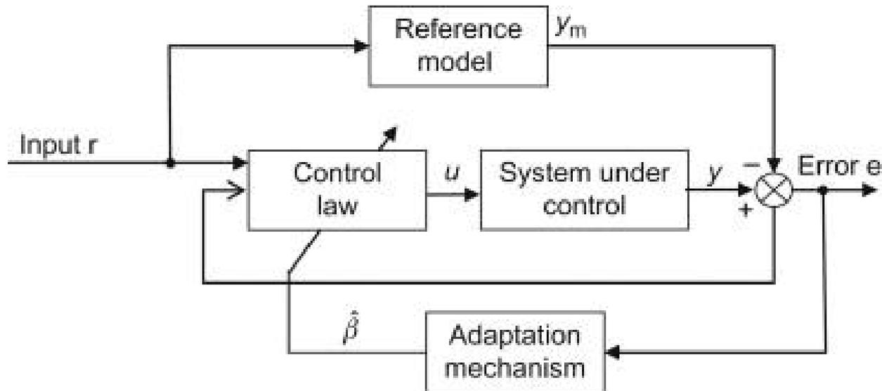
1. The system to be controlled that involves unknown parameters
