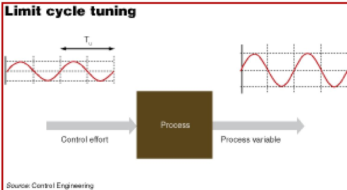
*Some self-tuning controllers wait for a limit cycle to occur before attempting to re-tune the loop. The current tuning parameters and the period of the limit cycle ( $T_u$ ) are all that's needed to re-tune the loop by the Ziegler-Nichols ultimate sensitivity method.*
