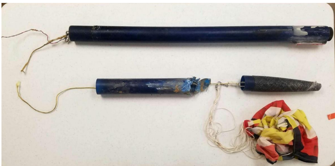
Figure 3.3.4b: Damages to the subscale rocket.
