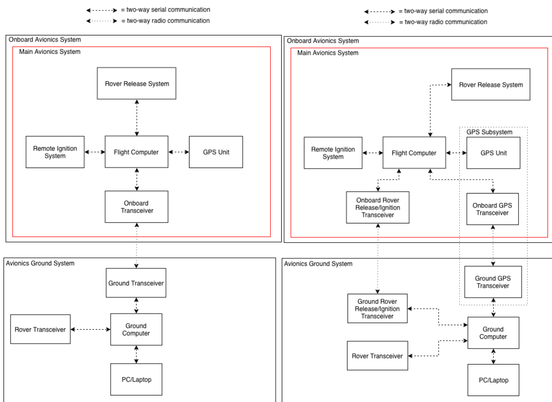
Figure 3.3.3b: Network diagram with one transceiver pair (left) and two transceiver pairs (right).
