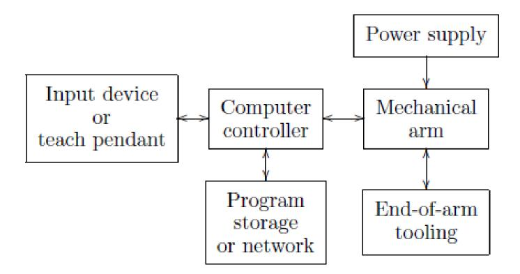
Figure 1.20: Components of a robotic system.
