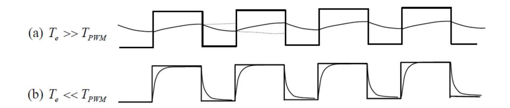
Figure: Current to the motor is smoothed due to the armature inductance L.
