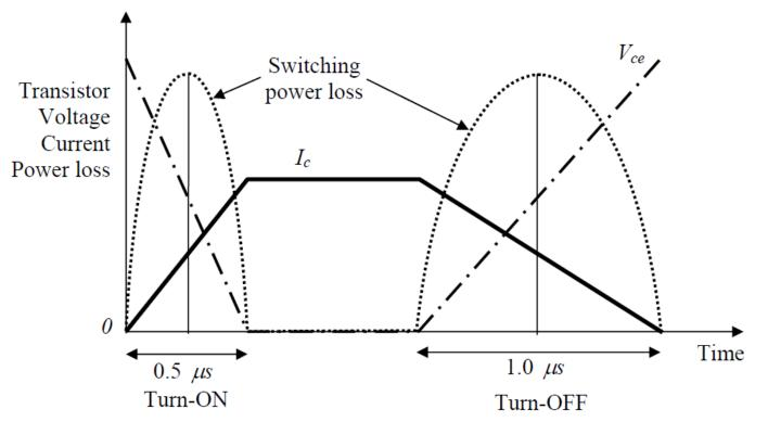
Transient responses of transistor current and voltage and associated power loss during turn-on and turn-off state transitions
