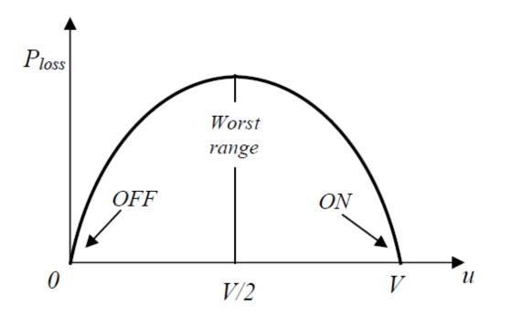
Figure: Power loss at the transistor vs. the armature voltage
