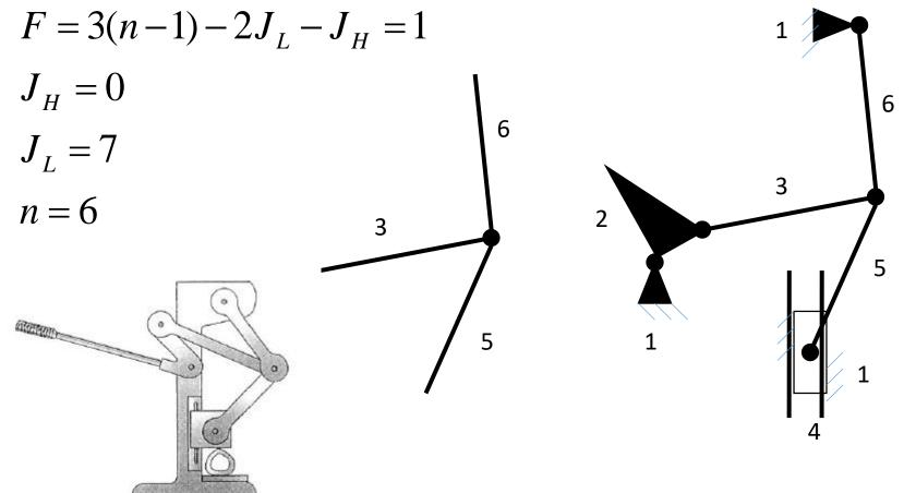
A joint with three concurring links can be decomposed as two revolute kinemamatic pairs
