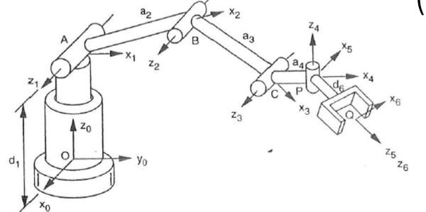
$$F = \lambda(n-1) - 5C_1 - 4C_2 - 3C_3 - 2C_4 = 30 - 25 = 5$$
