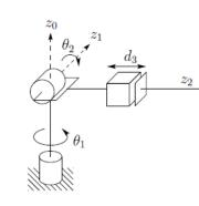
Figure 1.7: The spherical manipulator configuration.
