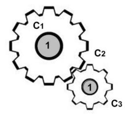
Gears are higher order kinematic pair, interacting by a contact point on the two active teeth.
