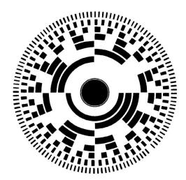
The disk is coupled to a motor shaft or a robot joint to measure. As it rotates, an **alternating ON-OFF** signal is obtained with the photodetector. <u>The number of grids passing through the optical elements represents the distance travelled.</u>
