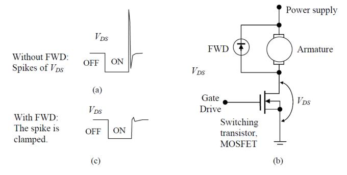
Voltage spike induced by inductance (a), free-wheeling diode (b), and the clamped spike with FWD (c)
