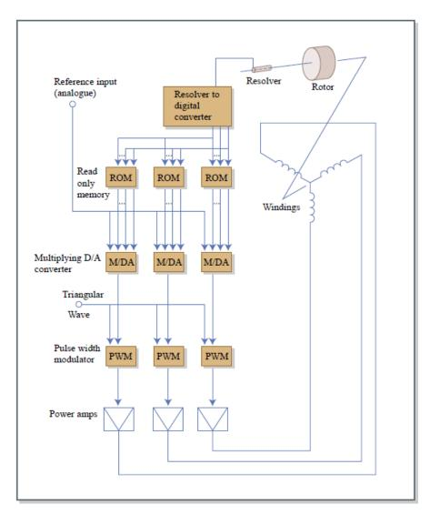
Let *I*<sub>A</sub>, *I*<sub>B</sub> and *I*<sub>C</sub> be individual currents flowing into the three windings (armatures) shown in the figure. These three currents are varies such that:
