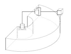
Figure 1.10: The SCARA (Selective Compliant Articulated Robot for Assembly).
