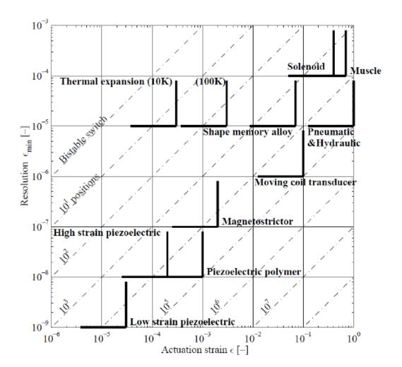
Strain resolution,  $\epsilon_{min}$ , versus actuation strain,  $\epsilon$ , for various actuators. Heavy lines bound the limits of performance.
