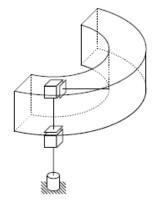
Figure 1.15: Workspace of the cylindrical manipulator.
