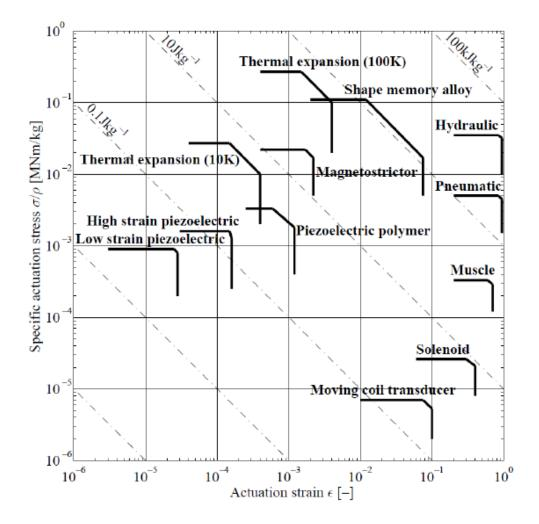
ecific actuation stress,  $\sigma/\rho$ , versus actuation strain,  $\epsilon$ , for various actuators. Heavy lines bound the upper limits of performance.
