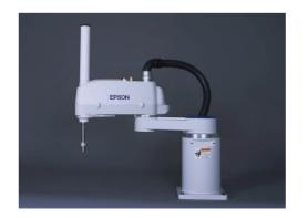
Figure 1.11: The Epson E2L653S SCARA Robot. Photo Courtesy of Epson.
