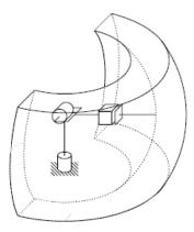
Figure 1.9: Workspace of the spherical manipulator.
