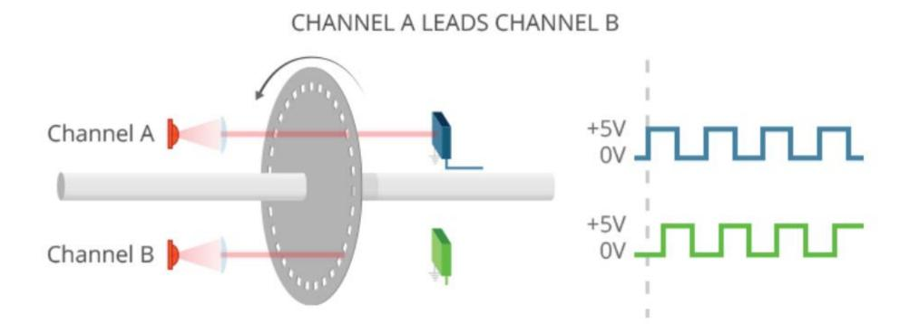
In this example, Channel A leads B, i.e., Channel A outputs a signal before Channel B. This indicates the shaft is rotating counter-clockwise.
