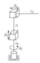
The cylindrical configuration is shown in Figure 1.13. The first joint is revolute and produces a rotation about the base, while the second and third joints are prismatic.
