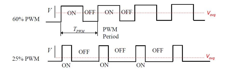
A single cycle of ON and OFF states is called the PWM period, whereas the percentage of the ON state in a single period is called *duty rate*.
