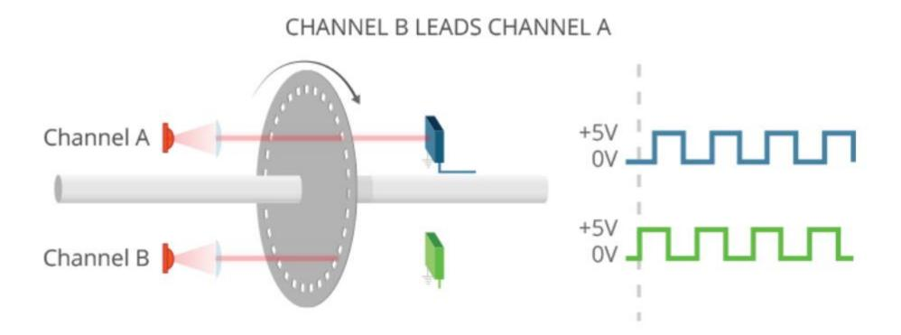
• In this example, Channel B leads A. This indicates the shaft is rotating clockwise.
