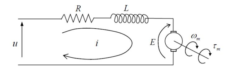
The actual DC motor is not a loss-less transducer, having resistance at the rotor windings and the commutation mechanism. Furthermore, windings may exhibit some inductance, which stores energy. Figure shows the schematic of the electric circuit, including the windings resistance R and inductance L. From the figure,
