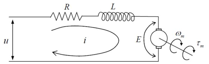
Electric circuit of armature
