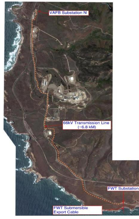
Figure 3-21. IDEOL FWT Substation and 66kV Transmission Line Route
