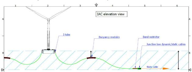
Figure 3-18. IDEOL Inter-Array Cable Elevation View
