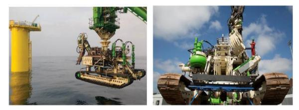
Figure 3-11. CADEMO Jet Trenching ROV (DEME Trenching Tool CBT1100)
