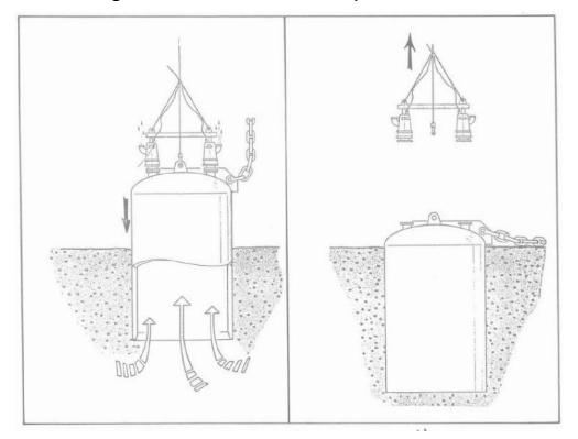
Figure 3-16. IDEOL Suction pile installation
