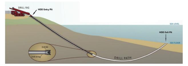
Figure 3-20. Conceptual Profile of an HDD Borehole
