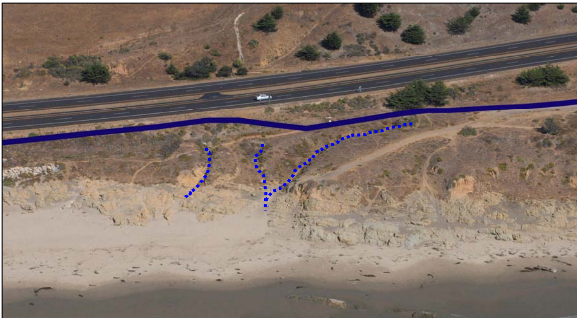
Figure 4.5-3 Incised Drainages at North Point Natural Area (in dashed blue)
