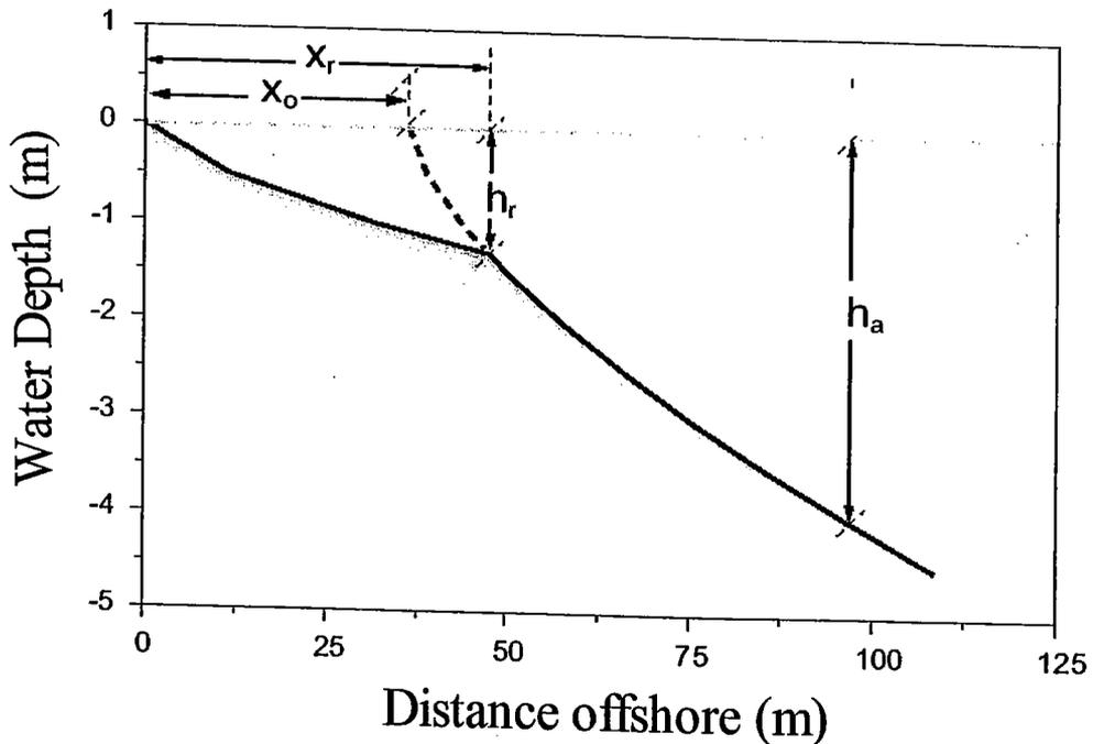
**Figure 1:** Definition sketch of surf and shoaling profiles. Surf profile extends from the shoreline to the breaking point. The offshore limit of the shoaling profile can be roughly estimated by,  $h_a \approx 3.5 H_s$  (Bernabeu, 1999)
