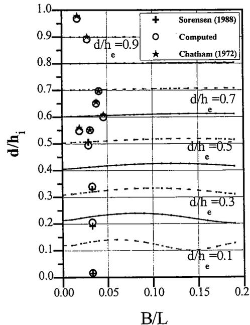
Figure 5. Numerical and experimental results of relative crest submergence,  $d/h_e$  versus relative width,  $B/L$  for different relative submergence,  $d/h_e$
