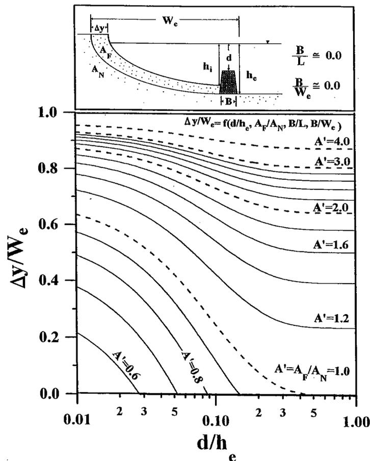
Fig. 5. Variation of non-dimensional shoreline advancement,  $\Delta y/W_e$  with  $A'$  and  $d/h_e$ . Results for  $B/L \cong 0.0$  and  $B/W_e \cong 0.0$ .
