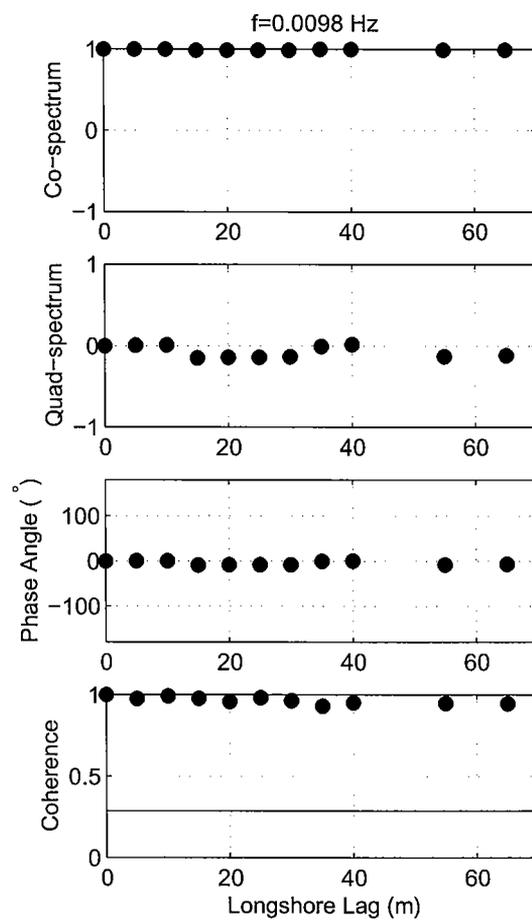
**Figure 12.** Co-spectrum, quad-spectrum, phase and coherence versus sensor separation for  $f=0.0098$  Hz. The spectra involve 56 degrees of freedom and a frequency bandwidth of  $1.95 \times 10^{-3}$  Hz.
