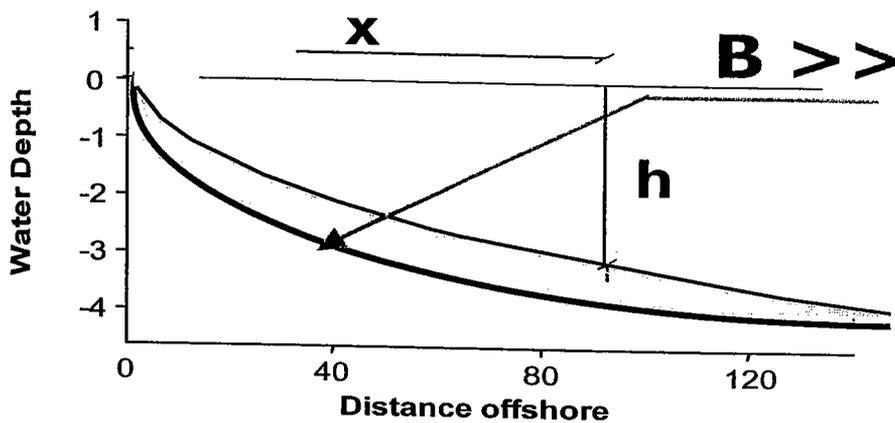
**Figure 4.** Influence of  $A$  and  $B$  parameters on the profile shape. Greater values of  $A$  and  $B$  increase shoreface slope and decrease submerged slope
