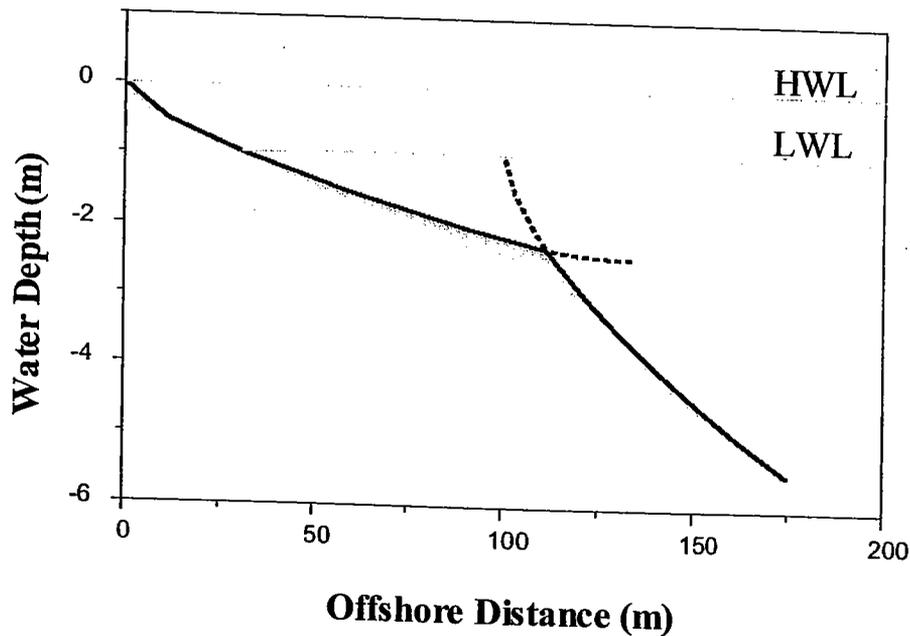
**Figure 5.** Definition sketch of EBP in a tidal sea. The main effect of the tide is that it acts as a stretching factor that increases the length of the breaking profile.
