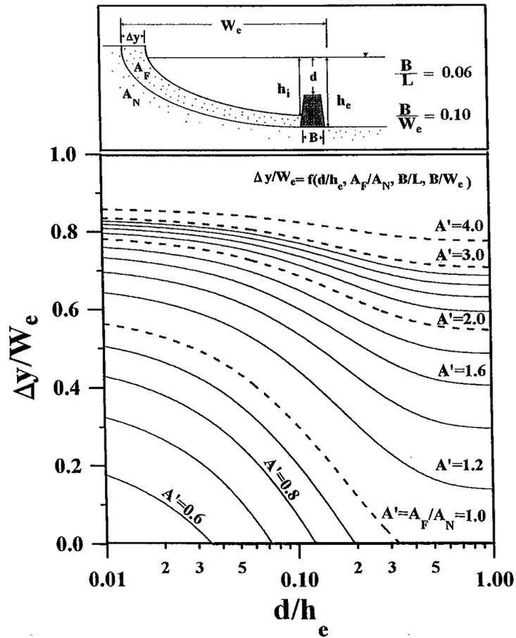
Fig. 6. Variation of non-dimensional shoreline advancement,  $\Delta y/W_e$  with  $A'$  and  $d/h_e$ . Results for  $B/L \cong 0.06$  and  $B/W_e \cong 0.10$ .
