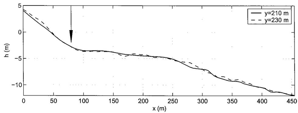
**Figure 3.** Cross-shore depth transects at longshore locations indicated by lines of corresponding type in Figure 2. The location of the longshore measurement array is marked with an arrow.
