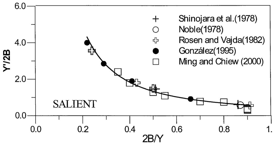
Figure 16. Relationship between the theoretical and the actual salient shape expressed in terms of  $Y$  and  $Y'$  (see figure 17). Dimensionless parameters,  $Y'/2B$  and  $2B/Y$  are used to fit the field and laboratory data presented in table 2. Equation 20 is also graphed (solid line).
