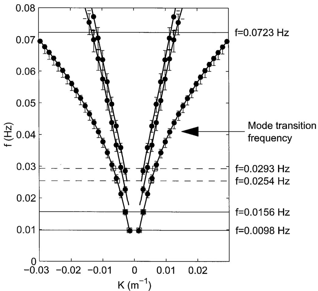
**Figure 19.** Theoretical edge wave resonances (bullets) and observed edge waves (squares). The mode transition frequency from cross-shore mode 0 to cross-shore mode 1 is also noted.
