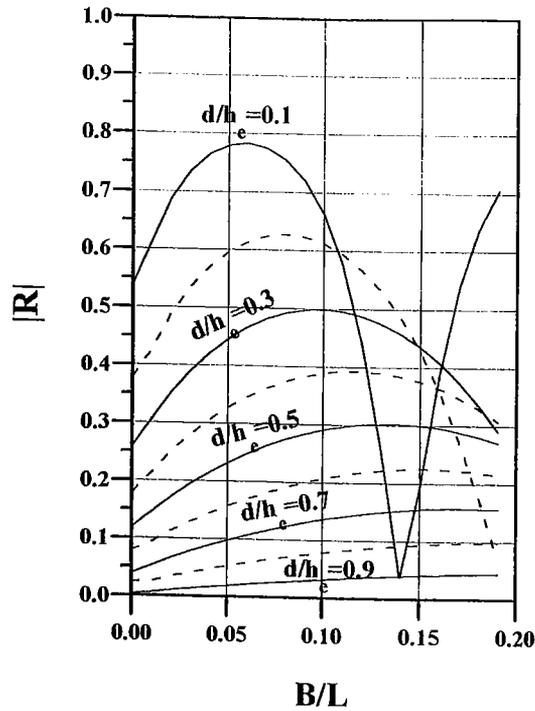
Fig. 3. Reflection coefficient  $R$  vs. relative width,  $B/L$  for different relative submergence of the breakwater,  $d/h_e$ . Notice that for any value of  $d/h_e$ , there is a value of  $B/L$  that yields no reflection so that all the energy flux is transmitted over the structure (resonant effect).
