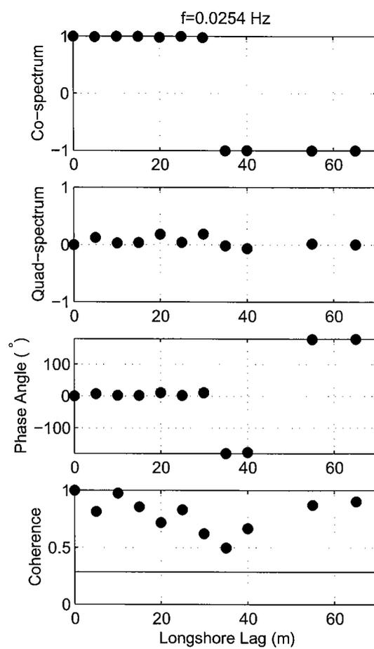
**Figure 14.** Co-spectrum, quad-spectrum, phase and coherence versus sensor separation for  $f=0.0254$  Hz. The spectra involve 56 degrees of freedom and a frequency bandwidth of  $1.95 \times 10^{-3}$  Hz.
