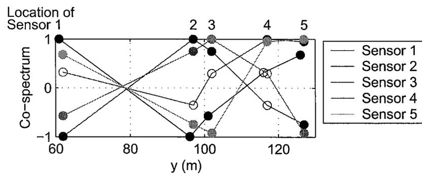
**Figure 18.** Co-spectrum, quad-spectrum, phase and coherence versus absolute sensor location for  $f=0.0723$  Hz. The spectra involve 56 degrees of freedom and a frequency bandwidth of  $1.95 \times 10^{-3}$  Hz.
