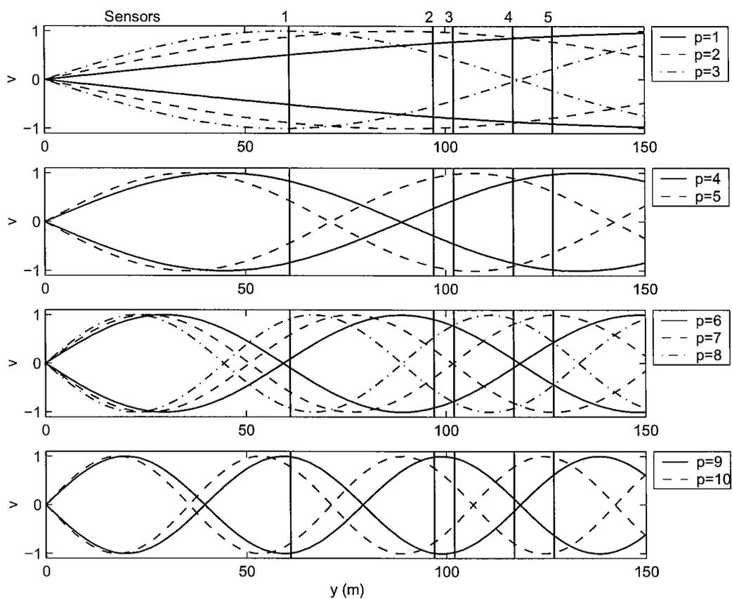
**Figure 8.** Theoretical nodal locations of the longshore velocity for several resonant edge wave modes. The vertical lines note the locations of the sensors.
