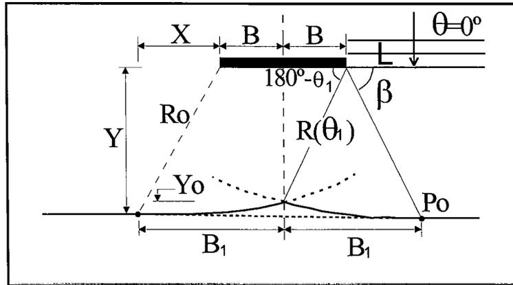
Figure 13. Definition sketch of a theoretical salient. The typical unknown variables, when designing a salient are the salient apex,  $Y_0$ , and the shoreline length affected by the breakwater,  $2B_1$ . These variables are given in figure 14.
