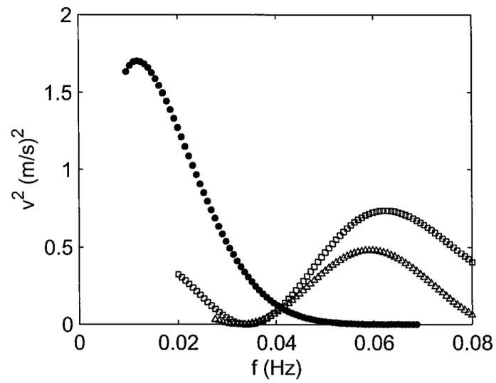
**Figure 5.** Simulated longshore velocity variance at the longshore array (located 35 m from the shoreline) as a function of frequency for edge waves with cross-shore mode number 0 (bullets), 1 (squares) and 2 (triangles).
