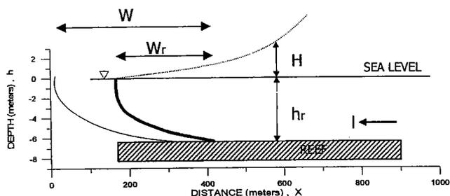
Figure 6. Definition sketch parameters for the reef-protected beach.
