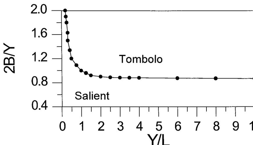
Figure 17. Proposed limiting condition for a tombolo or salient formation for a given length of the breakwater,  $2B$ , distance from the breakwater to the shoreline,  $Y$ , and wavelength,  $L$ . Note that for  $Y/L > 2.5$ , the curve slope is almost zero and, the limit for a tombolo formation is the only function of  $2B/Y \approx 0.86$  to  $0.88$ . However, for  $Y/L < 2.5$  the influence of  $Y/L$  must be taken into account.
