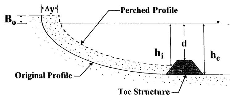
Fig. 1. Definition sketch of a perched beach. The main variables involved are the water depth over the breakwater,  $d$ , the water depth at the seaward and shoreward side of the toe structure,  $h_e$  and  $h_i$ , respectively, the advanced beach width,  $\Delta y$ , and the beach berm height,  $B_0$ .
