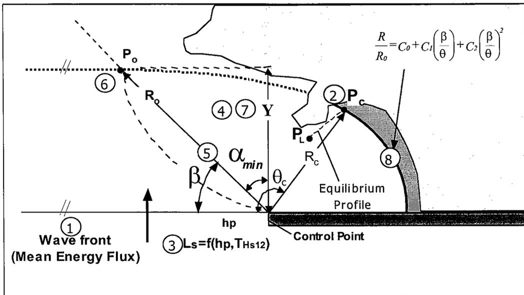
Figure 10. Definition sketch of the procedure method to test stability or to predict the static equilibrium shoreline in undeveloped bays. The numbers in the figure correspond to the different steps of the procedure.
