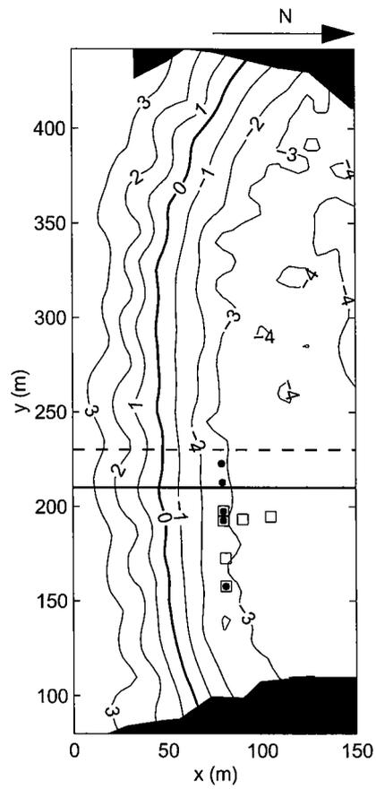
**Figure 2.** Measured bathymetry and instrument setup at Usgo beach. The available instruments were pressure sensors (squares), and bi-directional current meters (bullets). Also shown is the high tide shoreline (thick solid line).
