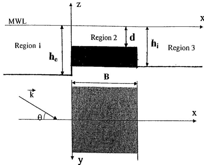
Fig. 7. Definition sketch of the rectangular impermeable step problem to be solved. One region is defined at each side of the step (regions 1 and 3) and another over the step (region 2). Incoming waves reach the step from region 1.
