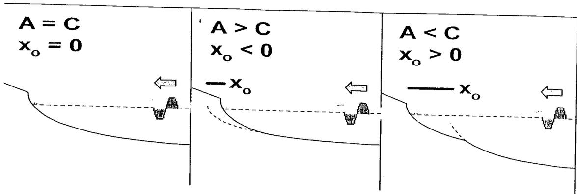
**Figure 2.** Definition sketch of profile offset,  $x_o$ , changes due to variation in  $A$  and  $C$ -parameters. If  $A$  is greater than  $C$ ,  $x_o$  is negative and the shoaling profile origin is located landward the breaking profile origin. For  $C$  values greater than  $A$ , the shoaling profile origin is located seaward the breaking profile origin.
