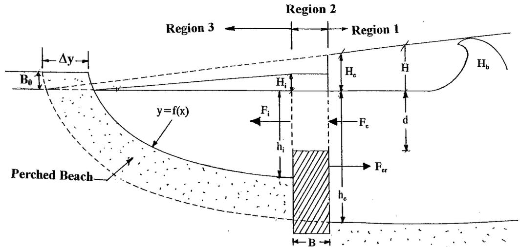
Fig. 2. Definition sketch of the three regions defined in order to solve the energy flux problem. Transmitted energy flux  $F_i$  and water depth at the shoreward side  $h_i$  are solved using an iterative process (Appendix A) and values of known data  $F_e$ ,  $d$ , and  $h_e$ .
