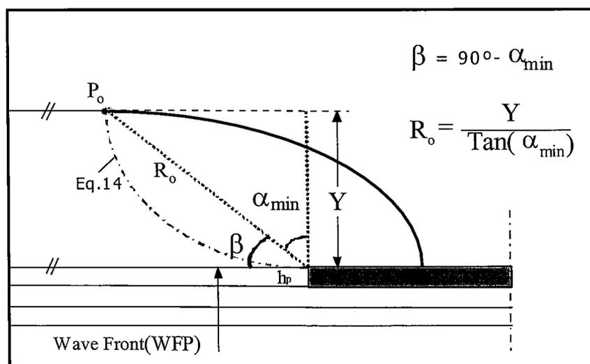
Figure 8. Definition sketch showing the relationship between the variables  $\beta$  and  $R_o$ , which are used in Hsu and Evans's (1989) equilibrium shape formulation (see also figure 1) and the variables  $\alpha_{min}$  and *Y* used in the proposed methodology. *Y* is the distance from the control point to the prolongation of the straight alignment downcoast.  $\alpha_{min}$  is related to  $\beta$  through  $\beta=90^\circ - \alpha_{min}$ .
