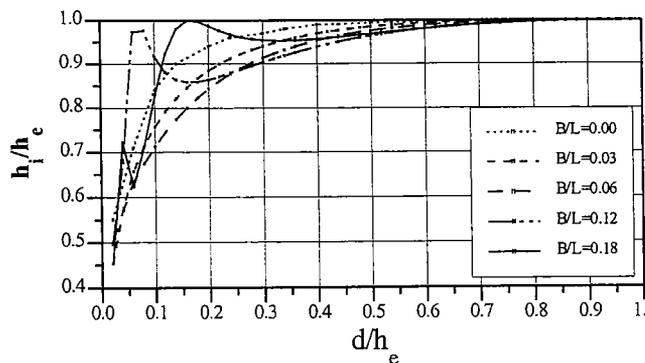
Figure 4. Relative depths  $h_i/h_e$  versus relative crest submergence,  $d/h_e$  for different relative width,  $B/L$ .
