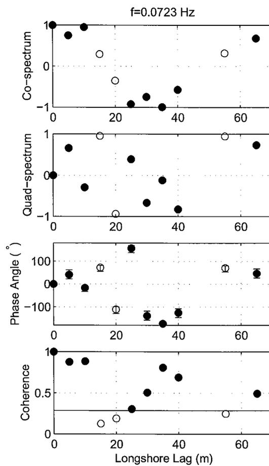
**Figure 17.** Co-spectrum, quad-spectrum, phase and coherence versus sensor separation for  $f=0.0723$  Hz. The spectra involve 56 degrees of freedom and a frequency bandwidth of  $1.95 \times 10^{-3}$  Hz.
