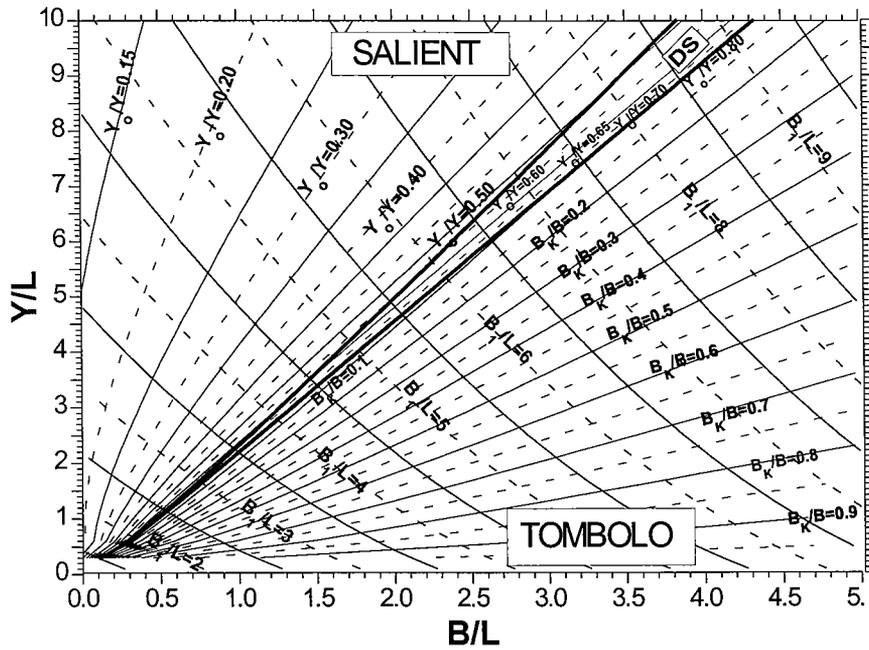
Figure 14. Variation of the non-dimensional equilibrium plan form parameters: for Tombolo: ( $B_k/B$ ,  $B_1/L$ ) and Salient ( $Y_0/Y$ ,  $B_1/L$ ) for different values of the length of the breakwater,  $2B$ , the distance from the breakwater to the shoreline,  $Y$ , and the wavelength,  $L$  (see figures 12 and 13 for a definition sketch of the different variables).
