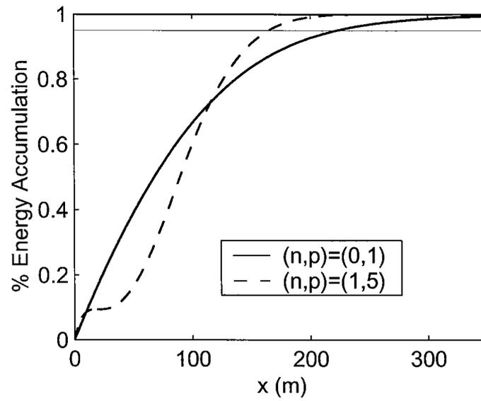
**Figure 7.** Energy accumulation of edge waves with  $(n, p) = (0, 1)$  and  $(n, p) = (1, 5)$ . 95% accumulation is also shown.
