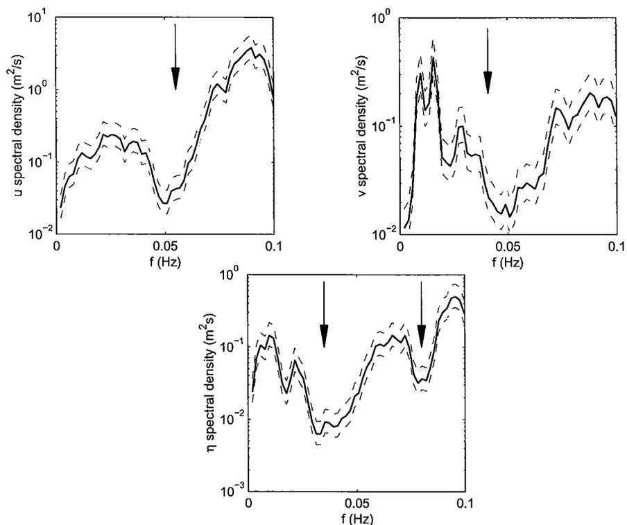
**Figure 10.** Frequency spectra of cross-shore velocity  $u$ , longshore velocity  $v$  and pressure  $p$  for sensor 3 (solid lines). The spectra involve 56 degrees of freedom and a frequency bandwidth of  $1.95 \times 10^{-3}$  Hz. The arrows indicate the locations of leaky wave zero-crossings for  $u$  and  $p$  and locations of mode transitions for  $v$ . The 95% confidence intervals are also shown (dashed lines).
