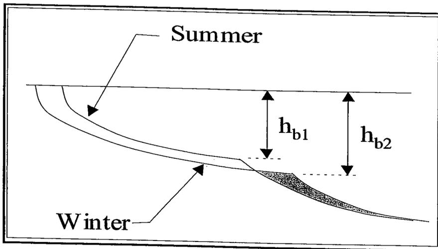
**Figure 3.** Definition sketch of seasonal beach changes due to variation in wave height. Changes in seasonal equilibrium are manifested by self-similar displacements of the two portions of the profile (surf and shoaling) as a consequence of changes in surf zone width and in the shape parameters
