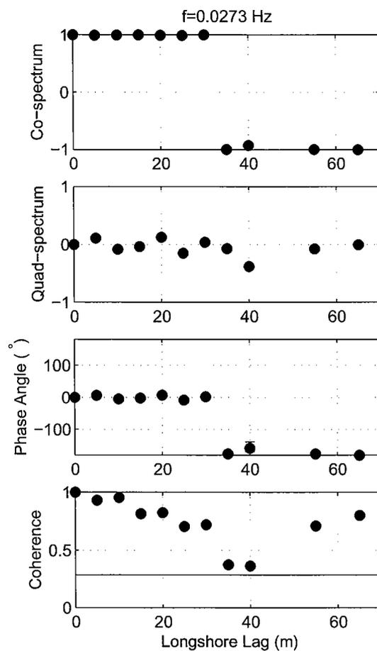
**Figure 15.** Co-spectrum, quad-spectrum, phase and coherence versus sensor separation for  $f=0.0273$  Hz. The spectra involve 56 degrees of freedom and a frequency bandwidth of  $1.95 \times 10^{-3}$  Hz.
