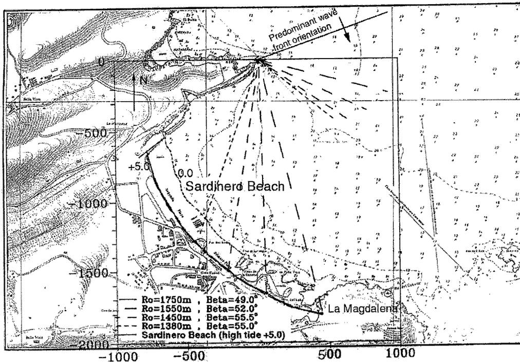
Figure 5. Predicted shorelines at Sardinero beach. Note that given a coastline point, the upcoast shoreline from that point can be represented using the tangent to the shoreline at that particular point as the orientation of the front at the diffraction point. In other words, any point can be used as the downcoast tip.
