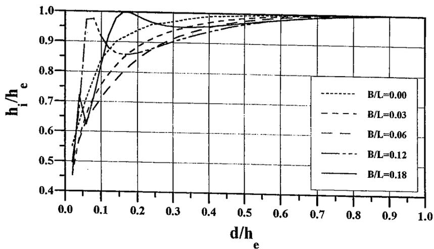
Fig. 4. Relative depths  $h_i/h_e$  vs. relative crest submergence,  $d/h_e$  for different relative width,  $B/L$ . Resonant effects are clearly observed for small  $d/h_e$  values and large values of  $B/L$ .
