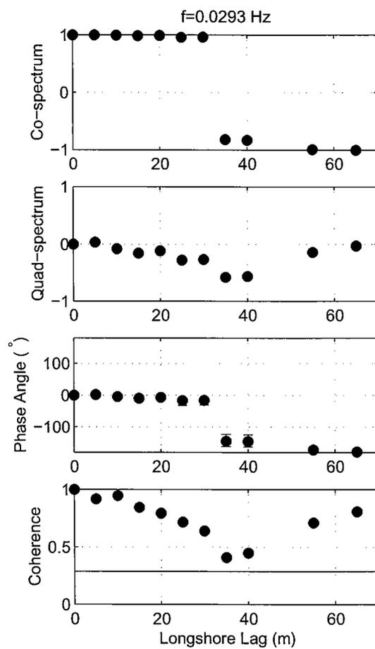
**Figure 16.** Co-spectrum, quad-spectrum, phase and coherence versus sensor separation for  $f=0.0293$  Hz. The spectra involve 56 degrees of freedom and a frequency bandwidth of  $1.95 \times 10^{-3}$  Hz.
