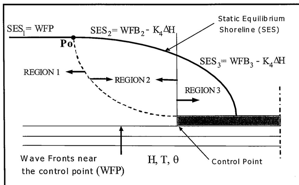
Figure 7. Definition sketch of the regions generated by an offshore barrier or breakwater. In region (1) the breakwater has no effect on the wave field, the wave height gradients are negligible and the wave fronts remain invariable; In region (2) wave height gradients are present and wave refraction is relevant; In region (3) wave height gradients and the turning of the fronts due to wave refraction-diffraction are important.
