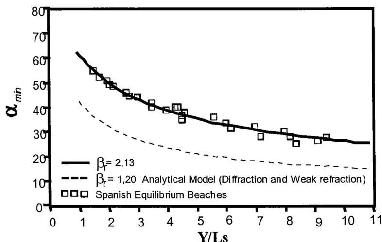
Figure 9. Value of the angle  $\alpha_{min}$  for different dimensionless distances from the control point to the prolongation of the straight alignment downcoast ( $Y/L$ ). These values have been obtained using data from 26 beaches along the Atlantic and Mediterranean coasts of Spain. The analytical expression for  $\alpha_{min}$ , for the case of diffraction with weak refraction derived by Gonzalez (1995) is also graphed with a dashed line.
