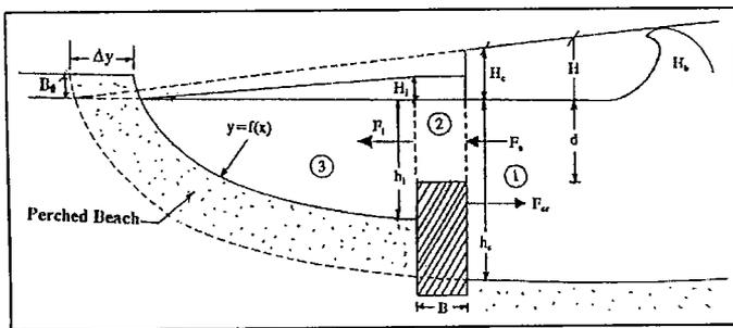
Figure 2. Definition sketch of parameters for the perched beach
