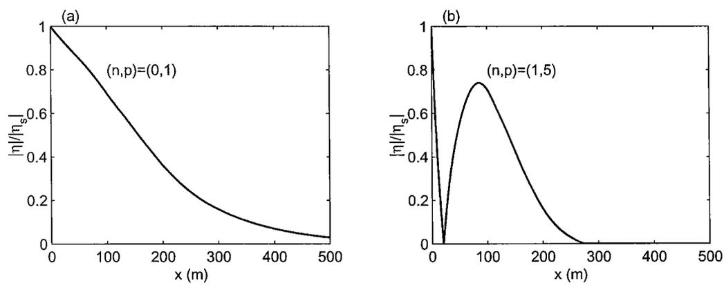
**Figure 6.** Simulated cross-shore profiles of the surface elevation due to edge waves for (a)  $(n,p) = (0,1)$  and (b)  $(n,p) = (1,5)$ .
