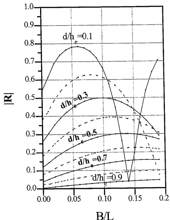
Figure 3. Reflection coefficient  $R$  versus width,  $B/L$  for different relative submergence of the breakwater,  $d/h_e$
