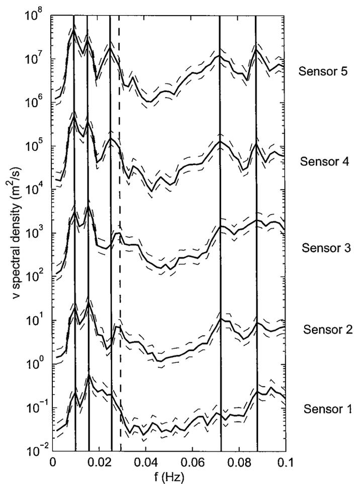
**Figure 11.** Frequency spectra of longshore velocities for sensors 1–5. Spectra have been multiplied by multiples of two orders of magnitude. The spectra involve 56 degrees of freedom and a frequency bandwidth of  $1.95 \times 10^{-3}$  Hz.
