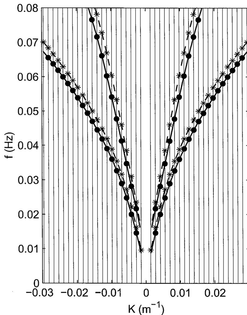
**Figure 4.** Dispersion lines for edge waves with cross-shore mode numbers  $n = 0$  and  $1$  for Usgo Beach at high tide (dashed line) and lowest tide (solid line) experienced during the four hours of data acquisition. Also noted are the theoretical edge wave resonances for a lateral beach width of 356 m for longshore mode numbers  $p$  1 through 21 for high tide (stars) and low tide (bullets). Note that the frequency  $f = 1/T$ , and the cyclic wavenumber  $K = 1/L$ .
