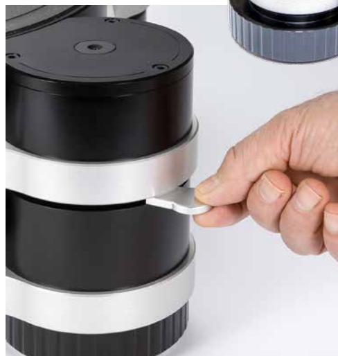
Flat shims provide the correct distance when adjusting the sub-chassis. If they just barely fit, the distance is correct.
