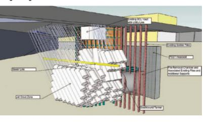
elevation 52 m (170 ft) to the base of the PSST structure. The layout of the piles avoids the electrical duct bank and the overhang of the existing vent structure.
