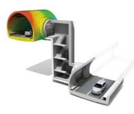
junction with super pile elements can be incorporated in one model file. Moreover, there are various types of interface elements, which enable the user to simulate soil-structure interaction regardless of the complexity of geometry and interface positions.
