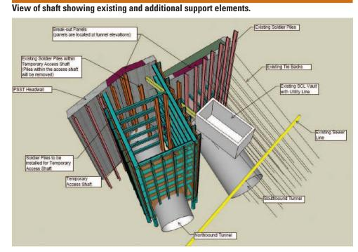
soldier piles within the shaft. • Upon completion of the works for the temporary pile removal chamber, the shaft will be excavated to a point where the northbound tunnel headwall break-out panel can be removed.
