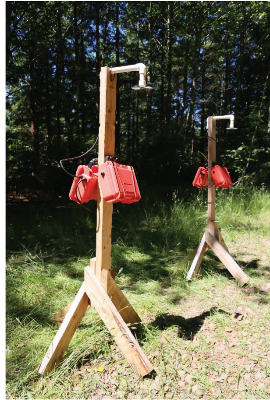
Figure 8. Running spore traps and batteries mounted on wooden frames. Photo by Miloň Dvořák.
