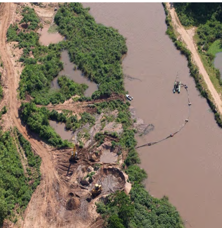
Various methods used to extract sand, including mechanical digging and dredging in the estuary (2019) Photo: Kierran Allen
