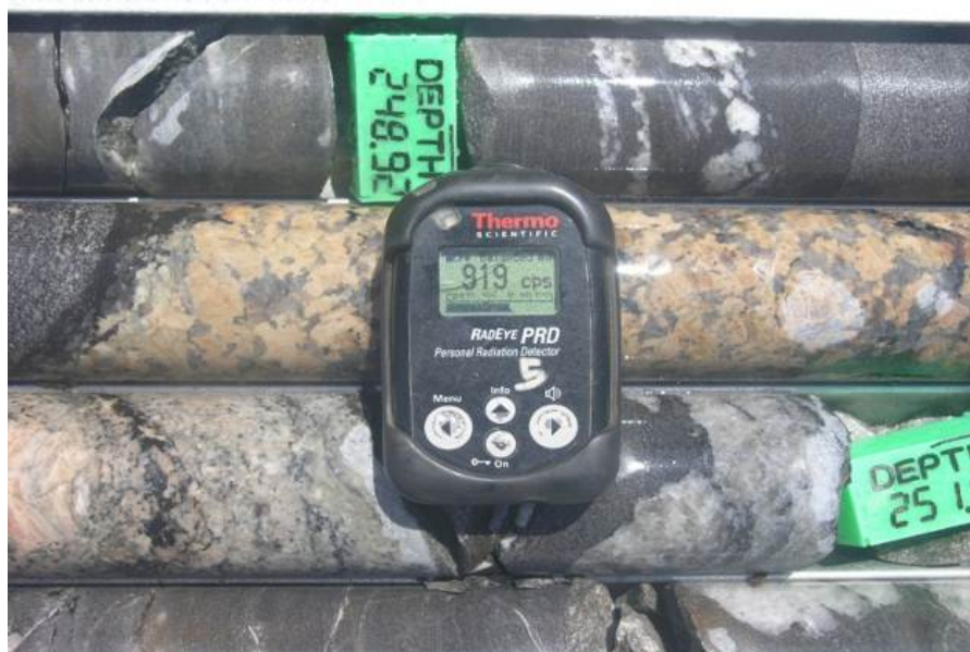
Figure 6.5 Ongolo Main (hole ALAD1557) - mineralised pegmatite within the Chuos formation at 249.70 m depth.
