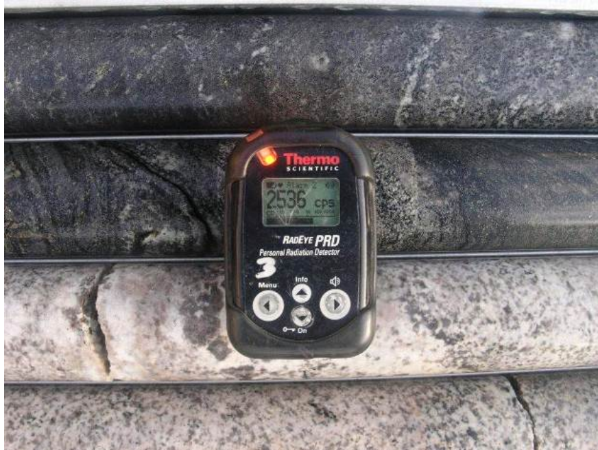
Figure 6.4 Ongolo Main (hole ALAD1553) - mineralised leucogranitic dyke within Chuos formation at 114.53 m depth.
