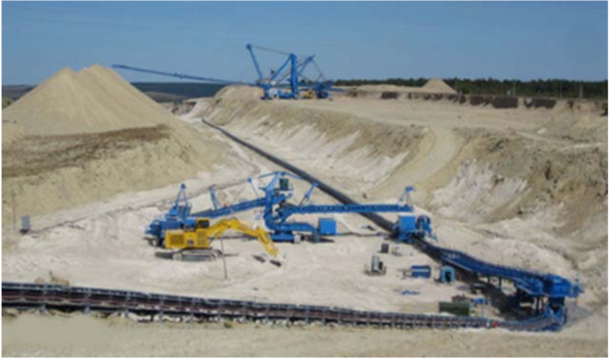
Figure 3.3 Schematic of an open cast mine employing in-pit crushing and conveying mining method.
