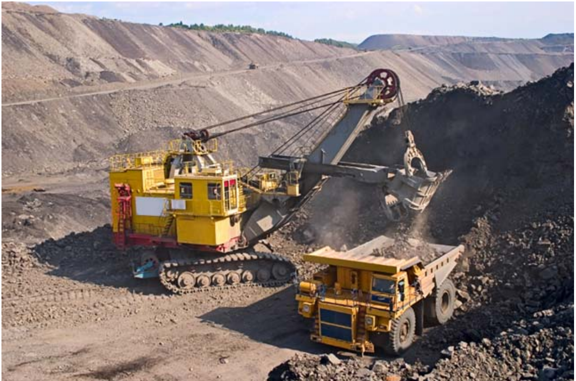
Figure 3.2 Open cast mining using excavator and haul truck mining method.
