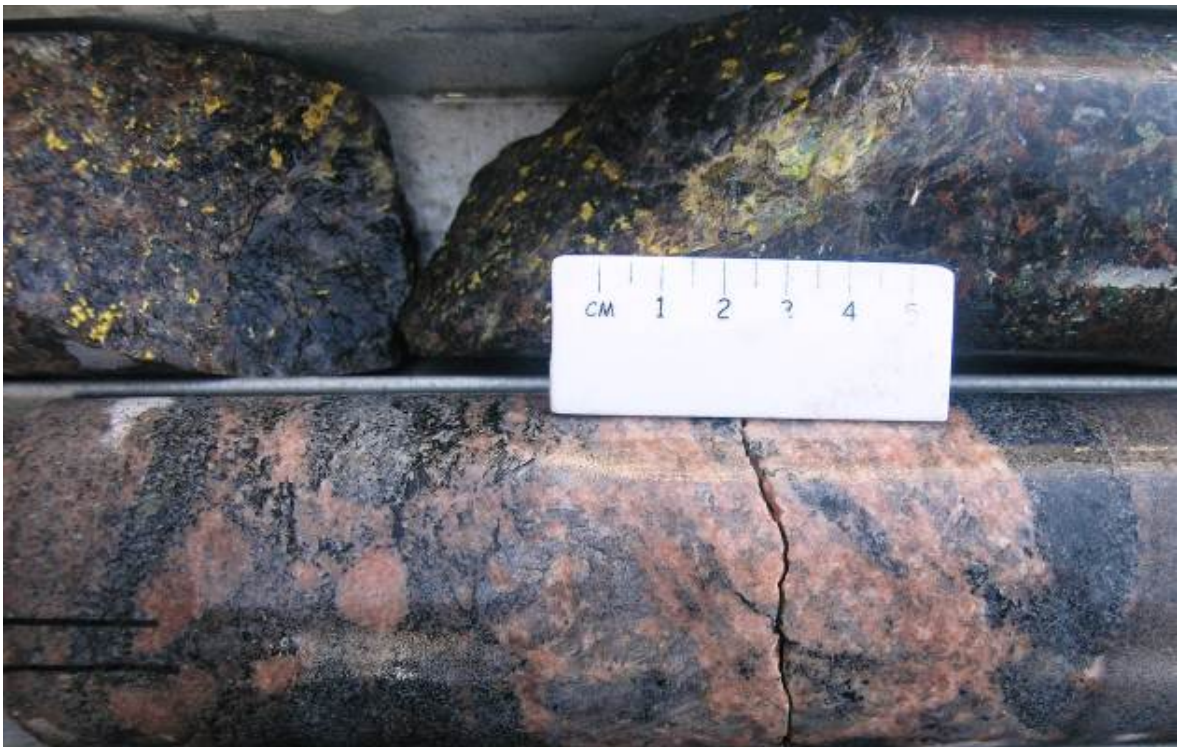
Figure 6.7 MS7 (hole ALAD1221) - uranophane in fractures zone at 173.5 m depth.
