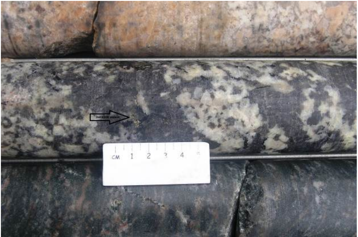
Figure 6.6 MS7 (hole ALAD1221) - mineralised granite with smoky quartz, biotite flakes and traces of secondary uranium mineralisation at 95.91 m depth.
