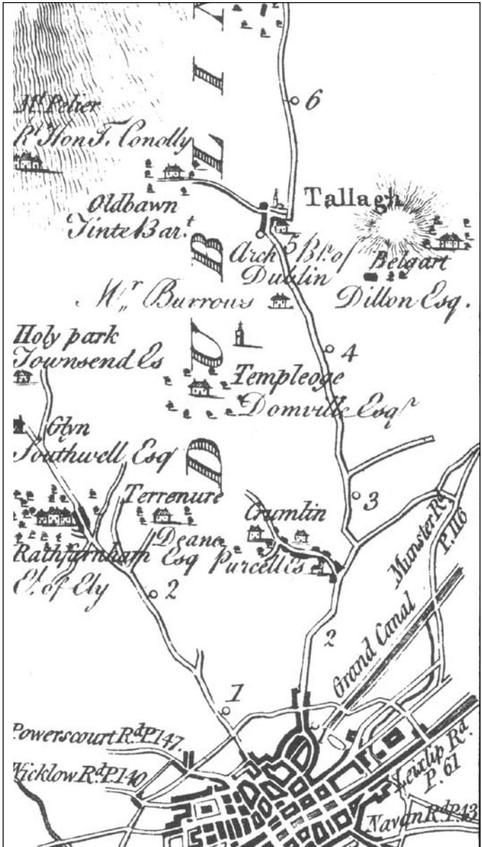
Portion of the map of the Road from Dublin to Tullow surveyed by Taylor and Skinner in 1777 showing the route along the Greenhills Road through Tallaght. The numbers along the road indicate the positions of Milestones.
