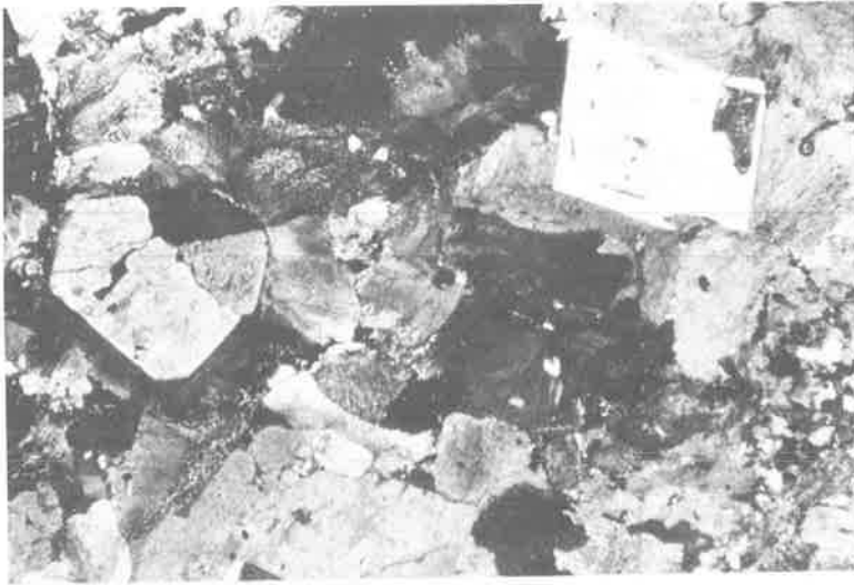
Figure 9. Photomicrograph of quartz and plagioclase phenocrysts set in the quartz-feldspar granophyric groundmass of a quartz keratophyre dike in the Roanoke Rapids complex. Outcrop is in the Roanoke River at Weldon, Weldon quadrangle.
