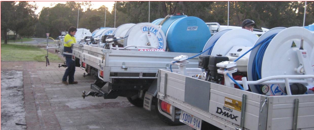
Figure 12: Vehicle mounted spray units are an effective means of applying foliar phosphite
