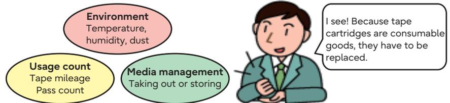
The lifespan of a tape cartridge varies depending on the usage environment, the number of times used, and the operation of the media, and it cannot be defined clearly. However, as the usage increases, the surface of the tape cartridge becomes damaged and the head becomes dirty causing an increase in read and write errors.
