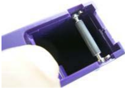
Figure A.4 Fit state of clips (clips do not fit correctly (the leader pin is misaligned))
