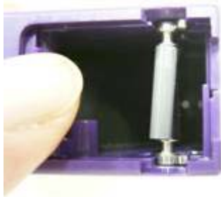
Figure A.4 Fit state of clips (clips do not fit correctly (the leader pin is misaligned))
