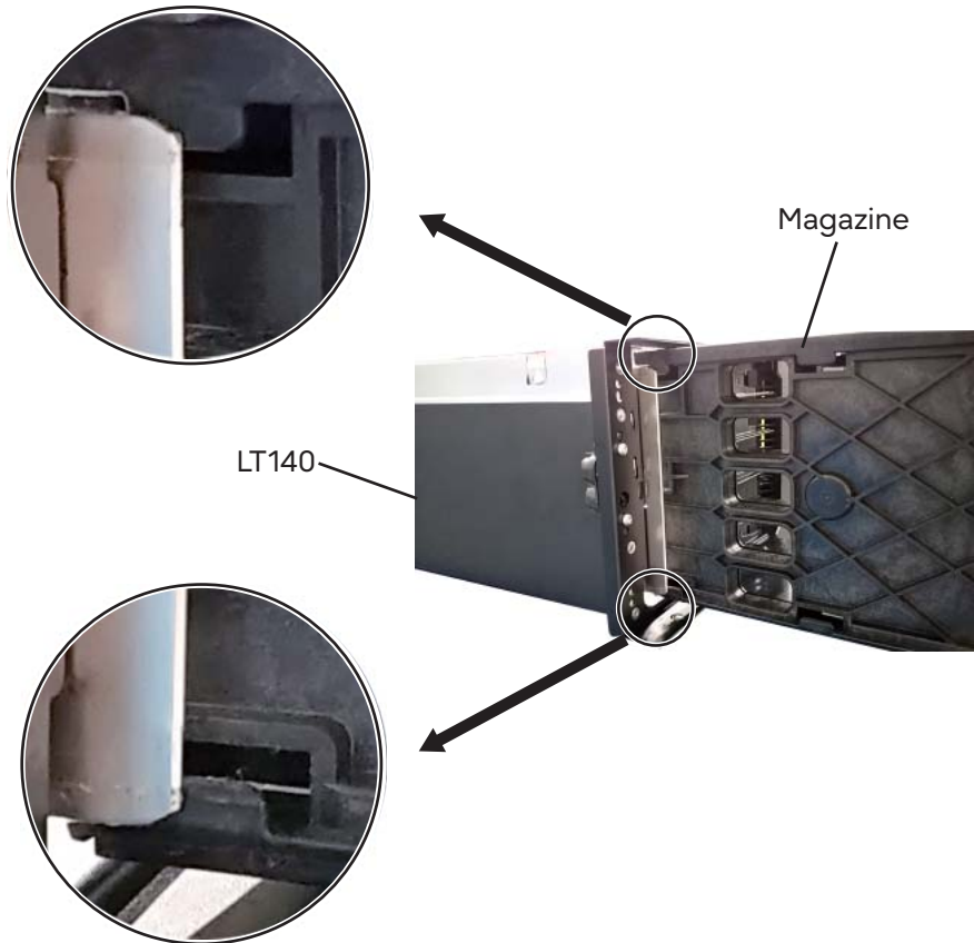
Figure 3.11 Inserting magazines (incorrect guide position)
