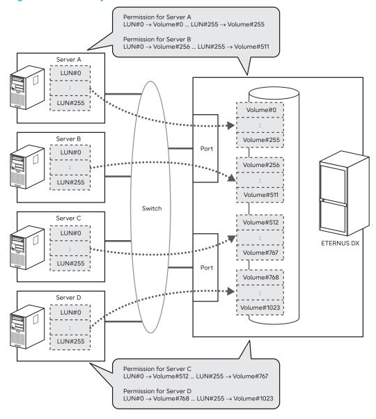
By using the host affinity function, a host interface port can be shared by multiple servers with different OSs in a system or by multiple servers in a cluster system.
