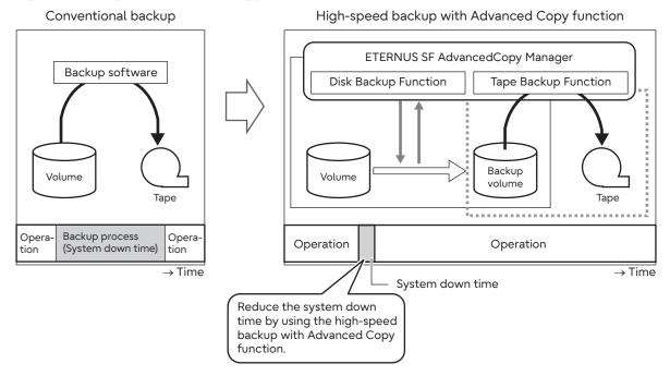
There are two types of Advanced Copy: a local copy that is performed within a single ETERNUS DX and a remote copy that is performed between multiple ETERNUS DX/AF storage systems.
