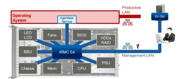
Fig. 12: ServerView out-of-band control – Concept
