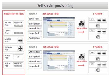
Fig. 10: Automated system provisioning from shared resources for multiple tenants
