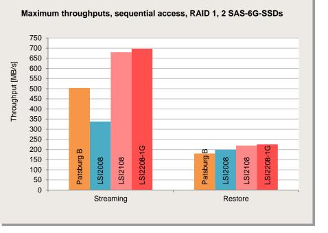
The Patsburg B controller achieves about 500 MB/s for the standard load profile "Streaming", which is equivalent to about twice the practical throughput limit of an SAS-3G connection. This means that the two SAS-3G connections are used to full capacity. The maximum sequential throughputs are achieved here with the LSI2108 and the LSI2208 controller. Both achieve throughputs of considerably more than 500 MB/s for the standard load profile "Streaming".
