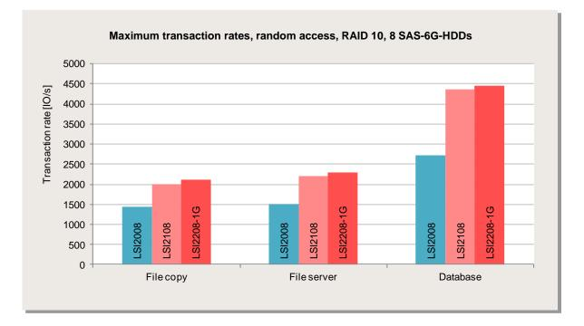
The diagram shows the same principal behavior as with RAID 0. This means that the controller without a cache (LSI2008) achieves at most about 70% of the transaction rate of the other two controllers with a cache for all the three load profiles depicted. Also for this RAID level this is a performance difference that only occurs above 32 parallel accesses to the RAID array.
