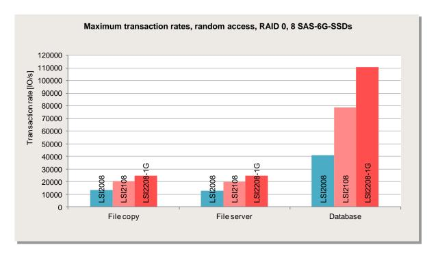
The LSI2208-1G controller is the one with top performance here.
