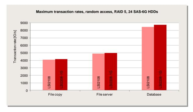
The LSI2208-1G controller, i.e. the newer controller with the larger cache, has a slight advantage.
