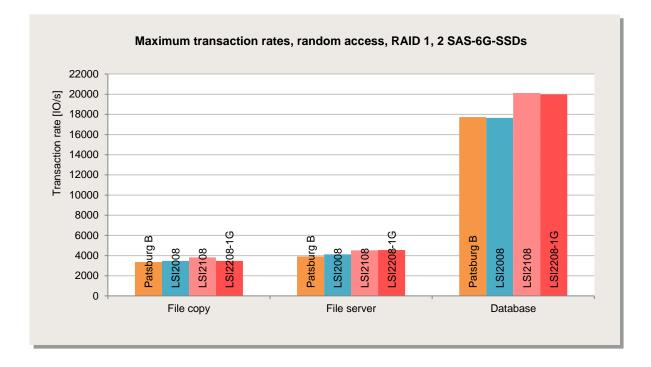
The LSI2108 and the LSI2208-1G controllers provide the highest overall transaction rates here.
