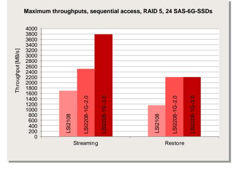
The great advantage of the LSI2208-1G-3.0 controller is clear to see here. As with RAID 0, 3800 MB/s are achieved with sequential read, which is clearly above the limit for PCIe Gen2.
