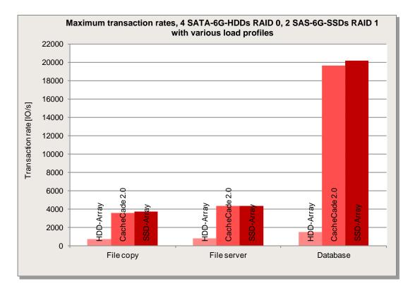
The measurement values refer to the LSI2208-1G controller. The HDD array consists of four SATA-6G-HDDs as RAID 0 and the CacheCade 2.0 cache consists of two SAS-6G-SSDs as RAID 1. The CacheCade 2.0 cache is configured for write and read. The maximum achievable transaction rates are shown in each case. A hot spot of 32 GB was assumed for access to the data.
