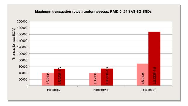
The LSI2208-1G controller is the one with top performance here. For the load profile with the smaller block size ("Database") it achieves approximately two and a half times the transaction rate of the LSI2108 controller.
