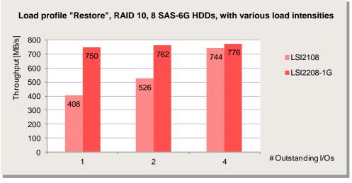
You can clearly see that in this case the LSI2108 controller does not achieve the same throughput for 1 and 2 outstanding IOs as the LSI2208-1G controller. The latter already achieves a throughput of 750 MB/s, whereas the LSI2108 controller only achieves a little more than half.
