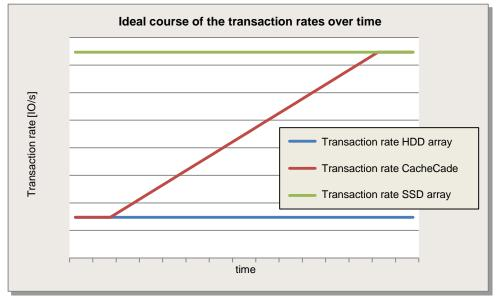
In relation to the SSDs the HDD array has a low transaction rate. During the data accesses the hot spot is gradually saved in the CacheCade 2.0 cache, which means on the SSDs, and you benefit from the relatively high transaction rate of the SSDs. Ideally, you achieve the transaction rate of a corresponding array consisting of SSDs.
