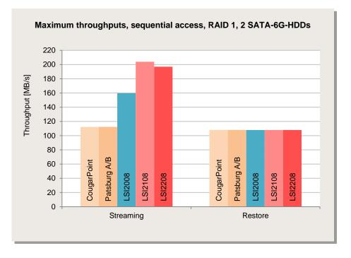
All in all, in the majority of cases for this RAID level the maximum throughputs are close to the maximum values of a single hard disk.
