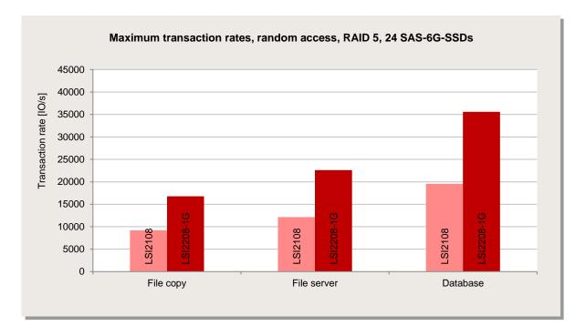
The technological progress from the previous to the current controller generation is as impressive here as in the case of RAID 0 with 24 SSDs: In the case of the standard load profile "Database" the LSI2208-1G controllers provide a transaction rate that is up to two times that of the LSI2108 controller.
