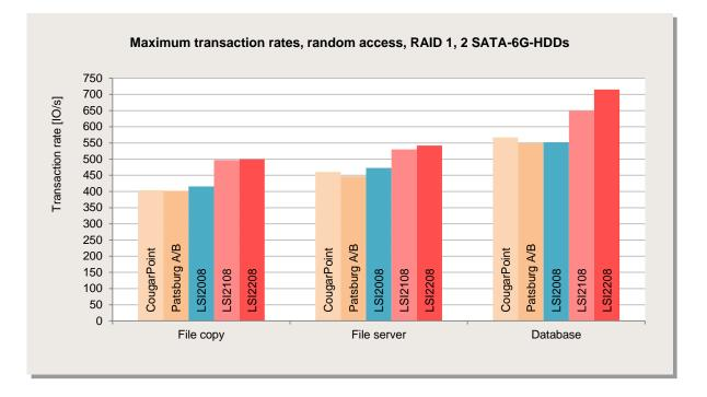
The LSI2108 and the LSI2208-1G controllers provide the highest overall transaction rates here.
