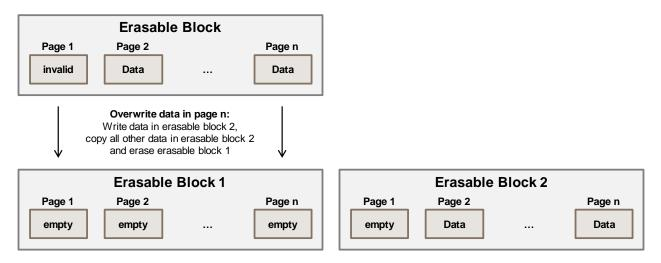
In this way, previously invalid pages are made available again for write jobs. This operation is called **garbage collection**. This ensures uniform wearing of the flash memory cells of pages that are updated (**dynamic wear-leveling**). To also enable the inclusion of flash memory cells of erasable blocks that are not updated in this wearing process, their data is also automatically moved at specific intervals (**static wear-leveling**).
