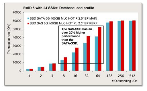
Database load profile (transaction processing): random, 67% read, 33% write, 8 kB block size
