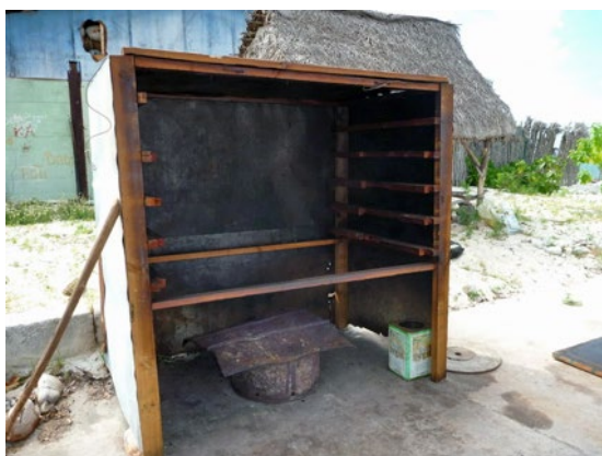
Figure 4. A smoke house on Tarawa, Kiribati, for smoking sea cucumbers. The sea cucumbers are placed on mesh trays that slide into the oven and sit well above a smouldering fire.
