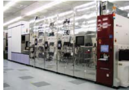
Immersion scanner & SOKUDO RF3S with integrated metrology (Photo Courtesy of IMEC)
