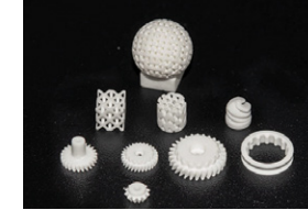
Micro 3D printed parts printed in AL Ceramic material
