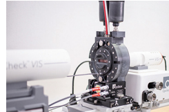
LensCheck™ and OpTest** Thermal Modules Test Lenses Across Temperatures from -40°C* to +120°C
