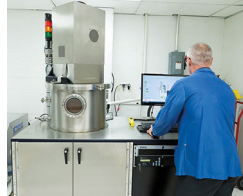
EMF's custom-designed DLC chamber eliminates pinholes, uniformity, stress, and adhesion in coatings
