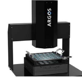
ARGOS matrix 200—The new industry standard for automated scratch-dig inspection
