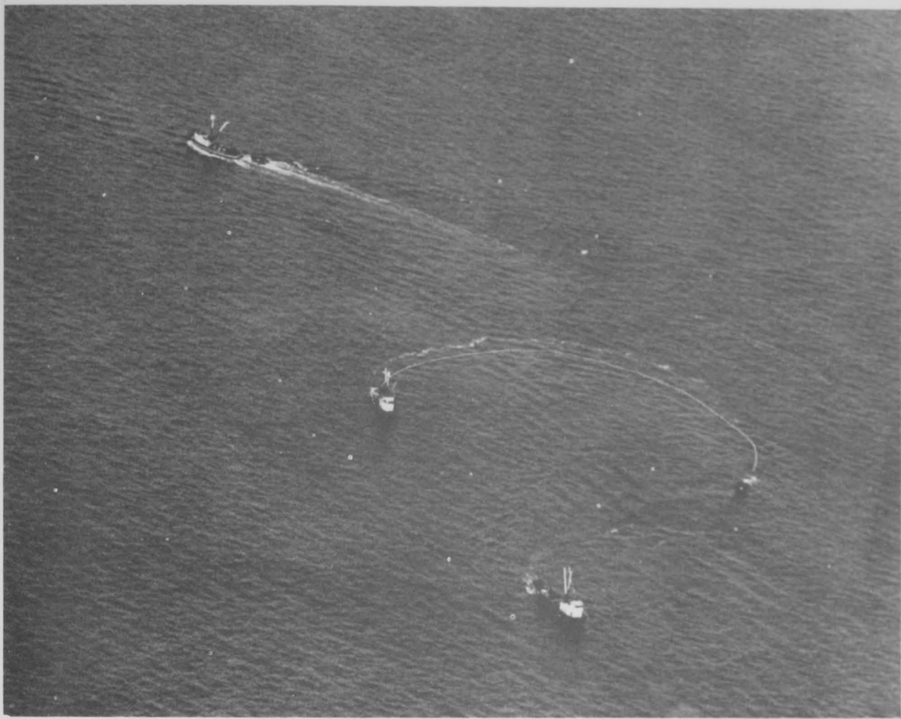
Figure 3.--View from airplane near Iquique, Chile. Vessel and skiff in center are setting the purse seine used to catch anchovy for reduction to meal and oil.
