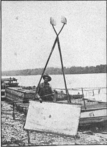
FIG. 1.—Shell tongs or scissors fork. The "mule" (in foreground) is not used with tongs, but in connection with crowfoot bars (in background). (See p. 56.)
