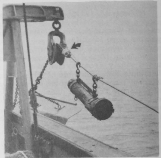
FIG. 2 - THE CUMBERSOME ACOUSTIC DEPTH TELEMETER UNIT, CENTER, HAS BEEN REPLACED BY THE SMALL ELECTRICAL DEVICE, UPPER LEFT, ATTACHED DIRECTLY TO THE END OF THE TRAWL CABLE.
