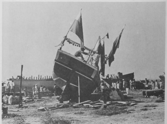
Fig. 10 - A new fishing vessel ready for launching in Karachi. It will be pushed, hauled, and lifted to the sea by about 100 men.
