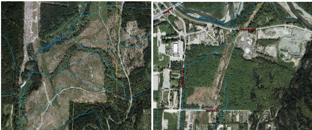
Figure 1. Aerial clip illustrating spatial inaccuracies of creek location versus on-the-ground watercourse location.
