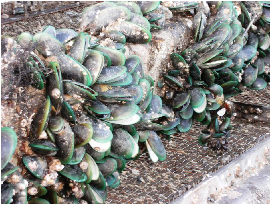
Fig. 3. Fouling of a power plant filter by Asian green mussels.
